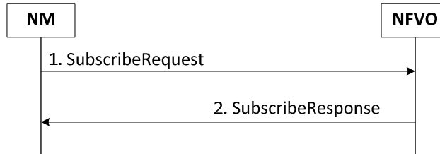
Figure 4.5.7-1: Subscribing to NSD change notifications through Os-Ma-nfvo
