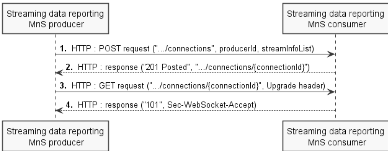
Figure 12.5.1.1.2-1: Message flow for establishing a streaming connection
