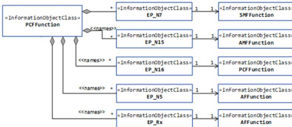
Figure 5.2.1.1-6: Transport view of PCF NRM
