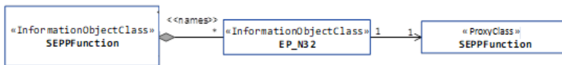
Figure 5.2.1.1-14: Transport view of SEPP NRM
