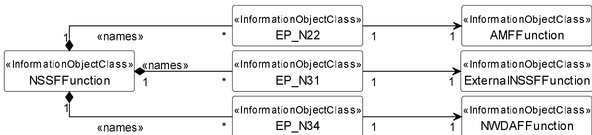
Figure 5.2.1.1-10: Transport view of NSSF NRM
