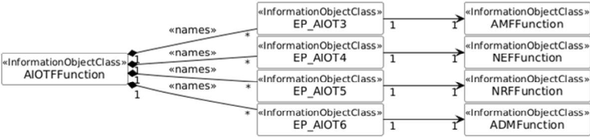
Figure 5.2.1.1-40: Transport view of AIOTF NRM
