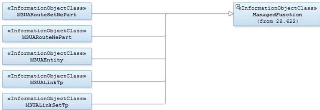
Figure 4.2.2-2: M3UA view of Signalling Transport Network Resource Model Inheritance Hierarchy
