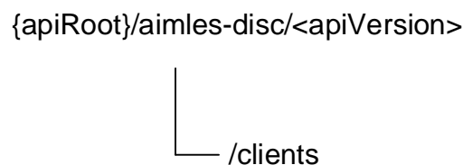
Figure 6.1.6.3.1-1: Resource URI structure of the AIMLES_AIMLEClientDiscovery Service API
