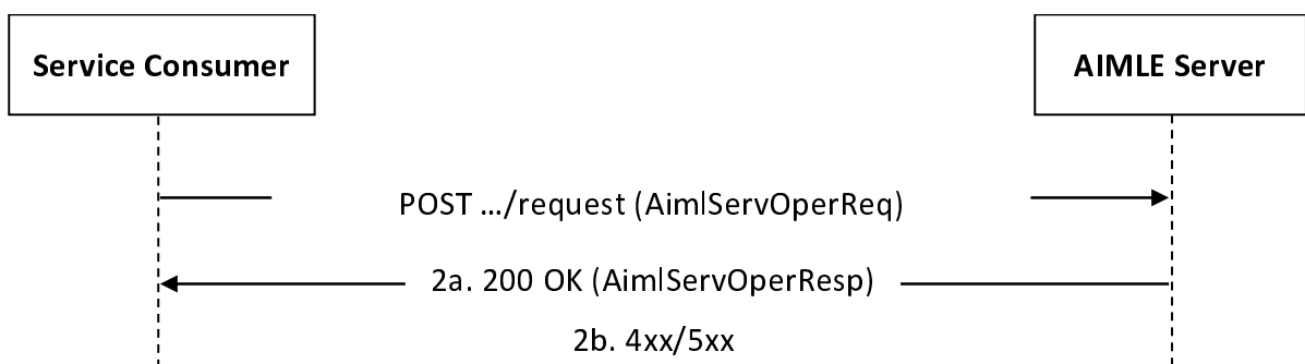
Figure 5.2.4.2.2.2-1: Procedure for AIMLE Service Operations Management Request
