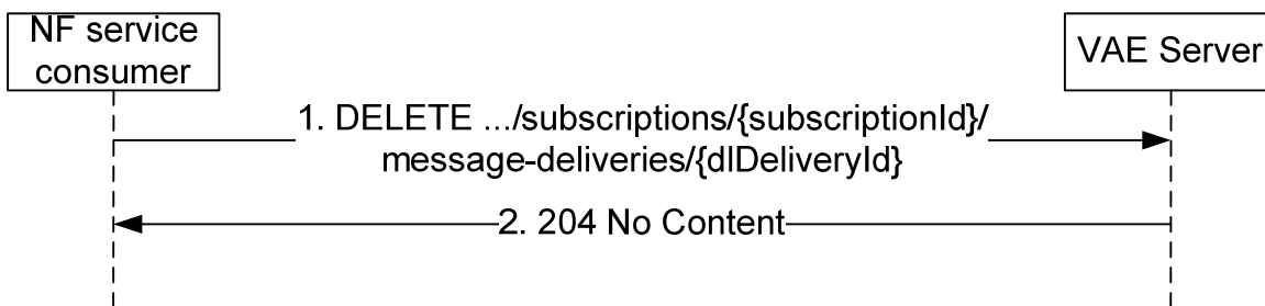
Figure 5.2.2.4.3-1: Termination of Downlink Message Delivery
