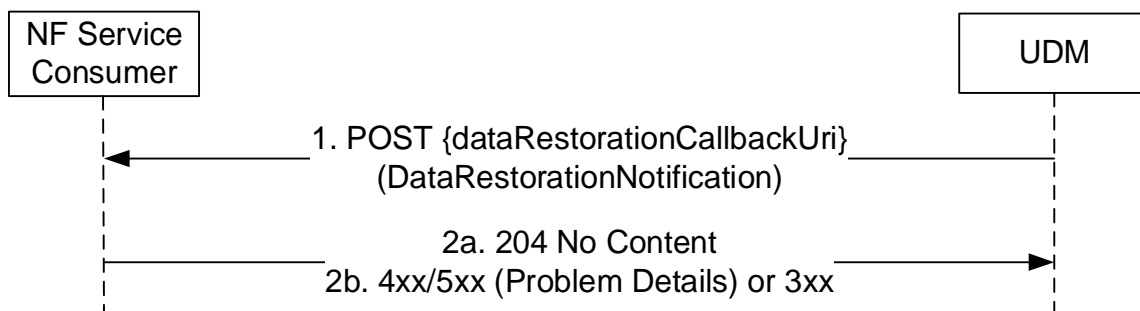
Figure 5.5.2.4.4-1: UDR-initiated Data Restoration
