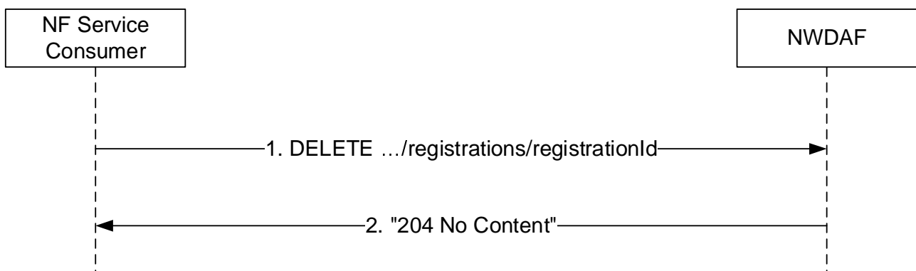
Figure 4.7.2.3.2-1: NF service consumer deregisters the use or monitoring capability of the analytics accuracy of an ML Model
