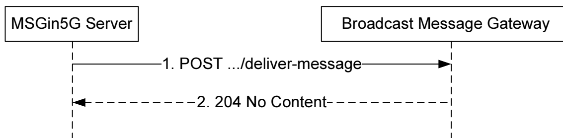
Figure 6.4.2.2.2-1: Broadcast Message Gateway Terminating Message Delivery
