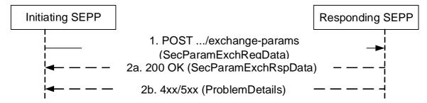
Figure 5.2.3.2-1: Parameter Exchange Procedure for Cipher Suite Negotiation
