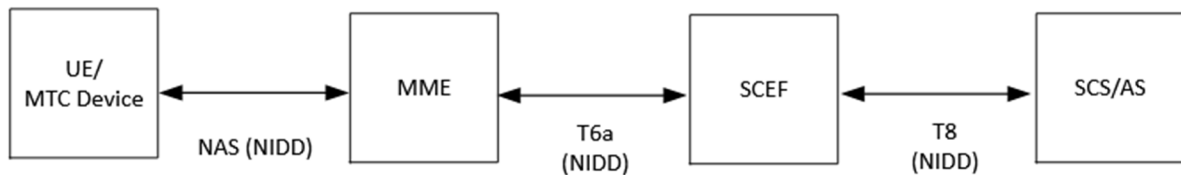
Figure 7.10.1.2.1-1: EPS Architecture for NIDD using SCEF
