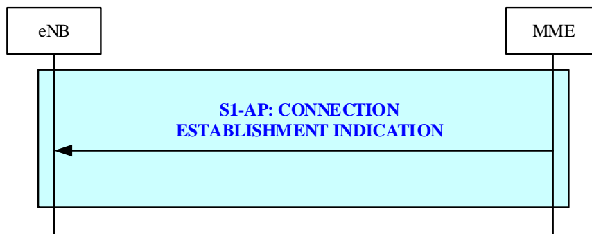
Figure 19.2.25-1: Connection Establishment Indication procedure
