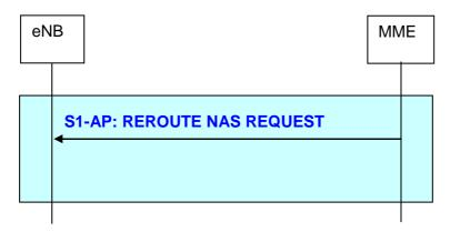
Figure 19.2.2.6-6: Reroute NAS Request procedure
