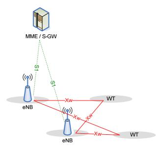
Figure 22A.1.1-1: Non-collocated LWA Overall Architecture
