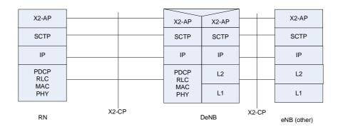
Figure 4.7.4-2: X2 control plane protocol stack for supporting RNs
