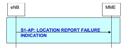
Figure 19.2.2.11.3-1: Location Report Failure Indication procedure
