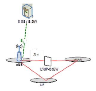
Figure 22A.3-1: LWIP Overall Architecture
