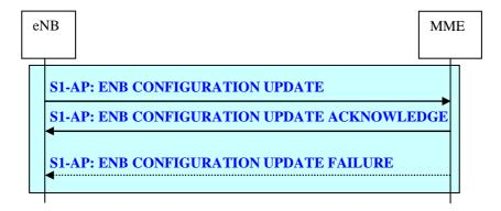
Figure 19.2.2.9-1: eNB Configuration Update procedure
