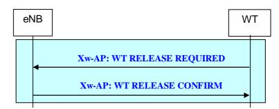
Figure 22B.2.2.6-1: WT initiated WT Release procedure
