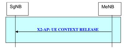
Figure 20.2.2.3-2: UE Context Release procedure for EN-DC.
