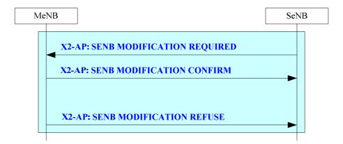
Figure 20.2.2.2d-1: SeNB initiated SeNB Modification procedure
