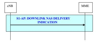
Figure 19.2.2.6-5: Downlink NAS Delivery Indication procedure
