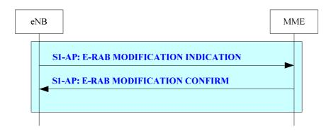
Figure 19.2.2.4.5-1: E-RAB Modification Indication procedure
