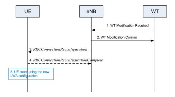
Figure 22A.1.7.2-2: WT Modification procedure - WT initiated
