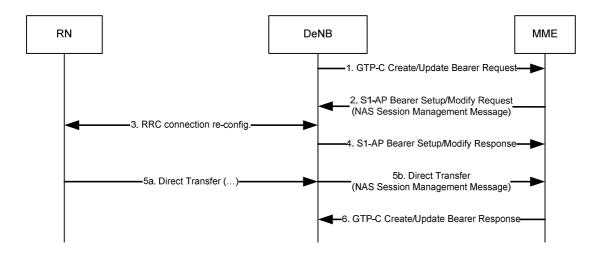
Figure 4.7.6.2-1: DeNB-initiated bearer activation/modification procedure
