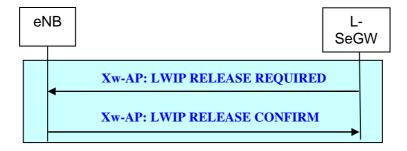
Figure 22B.2.2.16-1: LWIP-SeGW initiated LWIP-SeGW Release procedure
