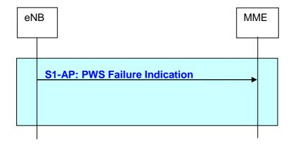
Figure 19.2.2.23-1: PWS Failure Indication procedure
