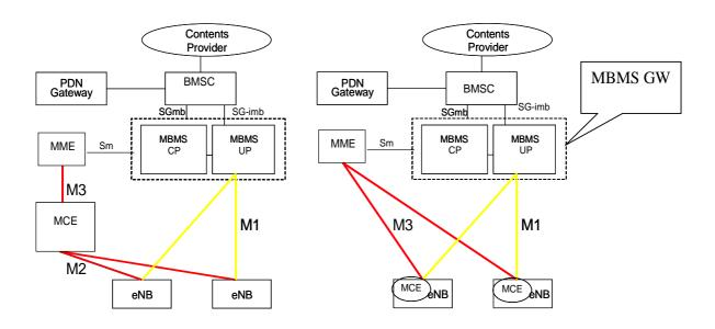
Figure 15.1.1-2: eMBMS Architecture deployment alternatives
