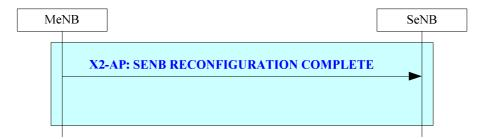
Figure 20.2.2.2b-1: SeNB Reconfiguration Completion procedure
