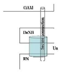
Figure 4.7.7.1-1: Relay OAM architecture.
