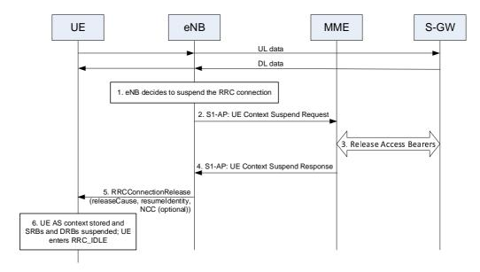
Figure 7.3a.3-1: RRC Connection Suspend procedure in EPS
