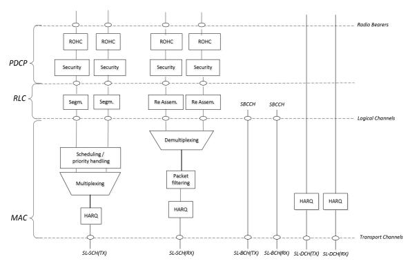
Figure 6-3: Layer 2 Structure for Sidelink
