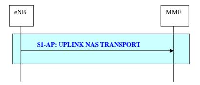
Figure 19.2.2.6-2: Uplink NAS Transport procedure
