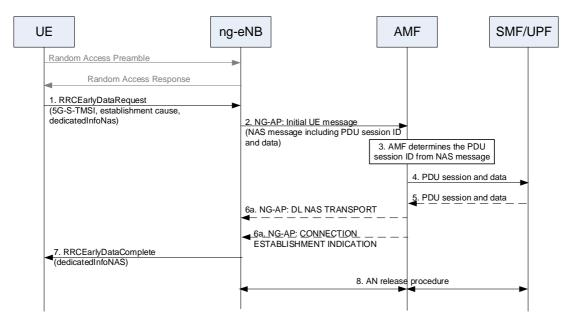
Figure 7.3b-1a: MO-EDT for Control Plane CloT 5GS Optimisation
