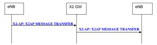
Figure 20.2.2.17-1: X2AP Message Transfer procedure
