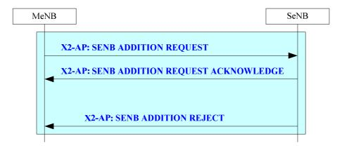
Figure 20.2.2.2a-1: SeNB Addition Preparation procedure
