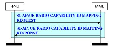
Figure 19.2.2.33-1: UE radio capability ID mapping procedure
