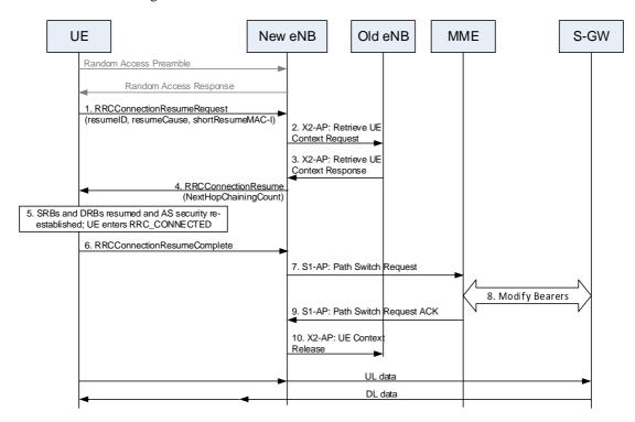
Figure 7.3a.3-3: RRC Connection Resume procedure in different eNB in EPS
