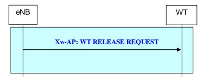
Figure 22B.2.2.5-1: eNB initiated WT Release procedure
