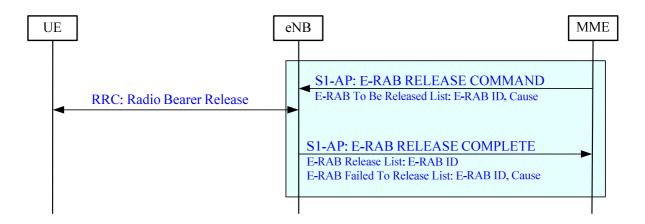
Figure 19.2.2.4.3-1: E-RAB Release procedure
