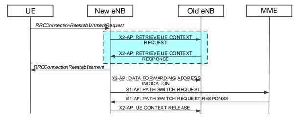
Figure 20.2.2.19-1A: Retrieve UE Context procedure (highlighted in blue) for cases of UE reestablishment. Successful case
