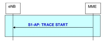
Figure 19.2.2.19.1-1: Trace Start procedure
