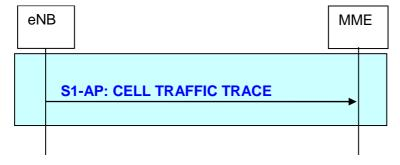
Figure 19.2.2.19.4-1: Cell Traffic Trace procedure
