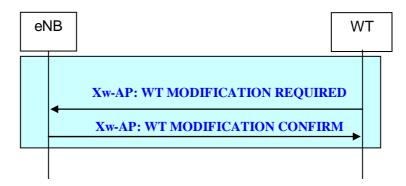
Figure 22B.2.2.4-1: WT initiated WT Modification procedure
