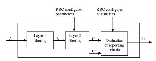
Figure 10.6-1: Measurement model
