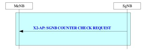
Figure 20.2.2.27-1: SgNB Counter Check procedure
