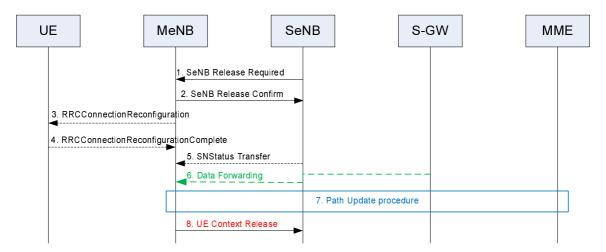
Figure 10.1.2.8.3-2: SeNB Release procedure – SeNB initiated
