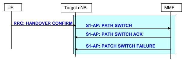
Figure 19.2.2.5.5-1: Path Switch procedure
