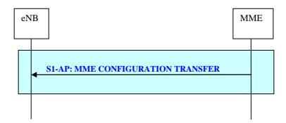
Figure 19.2.2.10a-1: MME Configuration Transfer procedure
