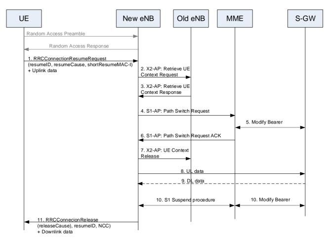
Figure: 7.3b-3: MO-EDT for User Plane CloT EPS Optimisations in different eNB
