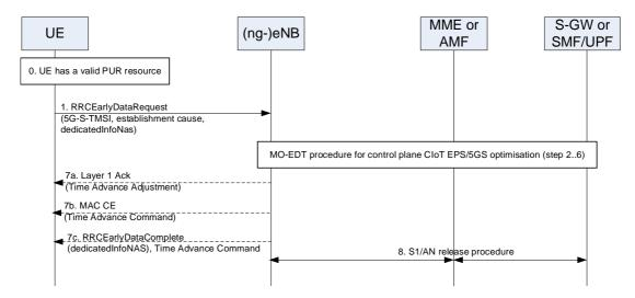
Figure 7.3d-2: Transmission using PUR for the Control Plane CloT EPS/5GS Optimisations
