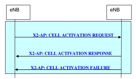
Figure 20.2.2.15-1: Cell Activation procedure
