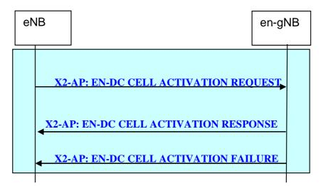
Figure 20.2.2.30-1: EN-DC Cell Activation procedure
