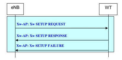
Figure 22B.2.2.9-1: Xw Setup procedure
