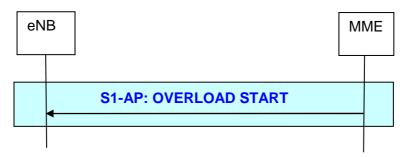
Figure 19.2.2.12.1-1 Overload Start procedure
