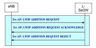
Figure 22B.2.2.13-1: LWIP-SeGW Addition Preparation procedure
