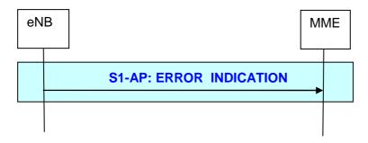
Figure 19.2.2.7.2a-1: eNB initiated Error Indication procedure
