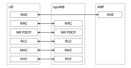
Figure 24.2.2-1: Control Plane Protocol Stack
