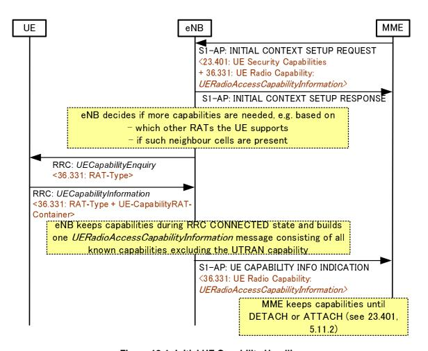
Figure 18-1: Initial UE Capability Handling
