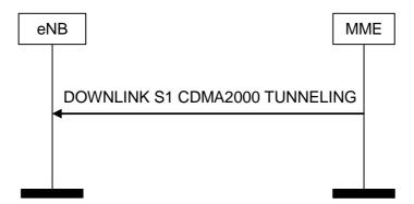
Figure 19.2.2.16.1-1: Downlink S1 CDMA2000 Tunnelling procedure
