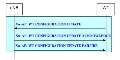
Figure 22B.2.2.10-1: WT Configuration Update procedure
