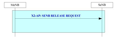
Figure 20.2.2.2e-1: MeNB initiated SeNB Release procedure
