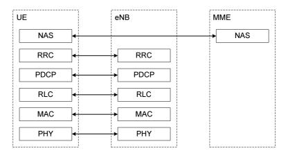
Figure 4.3.2-1: Control-plane protocol stack
