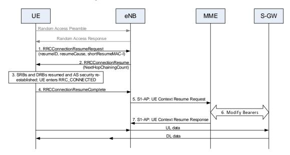
Figure 7.3a.3-2: RRC Connection Resume procedure in EPS
