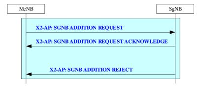
Figure 20.2.2.20-1: SgNB Addition Preparation procedure
