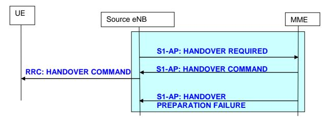
Figure 19.2.2.5.1-1: Handover preparation procedure
