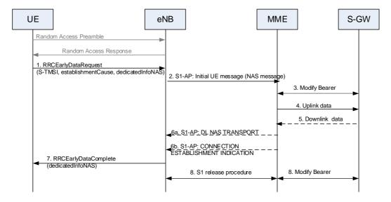
Figure 7.3b-1: MO-EDT for Control Plane CloT EPS Optimisation
