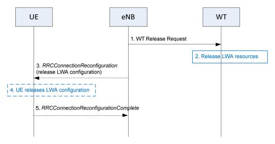
Figure 22A.1.7.3-1: WT Release procedure -eNB initiated
