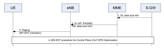
Figure 7.3c-1: MT-EDT for Control Plane CloT EPS Optimisation
