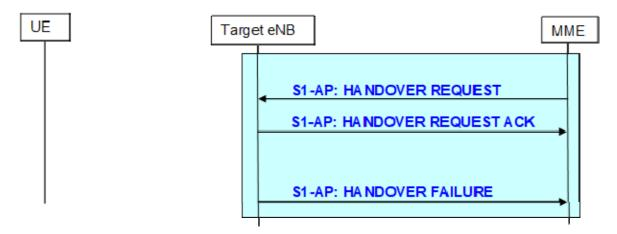
Figure 19.2.2.5.2-1: Handover resource allocation procedure
