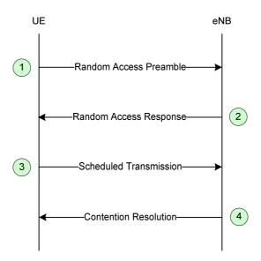
Figure 10.1.5.1-1: Contention based Random Access Procedure
