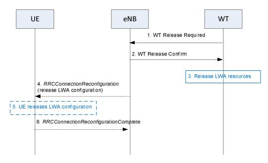
Figure 22A.1.7.3-2: WT Release procedure -WT initiated
