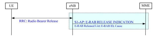
Figure 19.2.2.4.4-1: E-RAB Release Indication procedure
