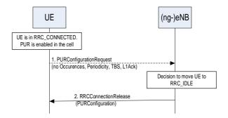
Figure 7.3d-1: PUR Configuration Request and PUR Configuration
