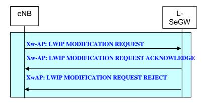
Figure 22B.2.2.14-1: eNB initiated LWIP-SeGW Modification Preparation procedure
