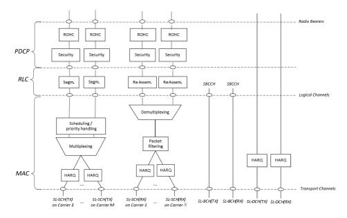
Figure 6.4-3: Layer 2 Structure for Sidelink with CA configured
