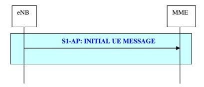
Figure 19.2.2.6-1: Initial UE Message procedure
