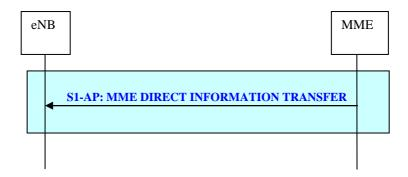
Figure 19.2.2.15-1: MME Direct Information Transfer procedure
