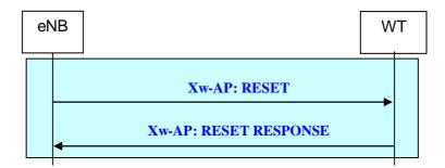
Figure 22B.2.2.12.2-1: Reset procedure initiated by eNB
