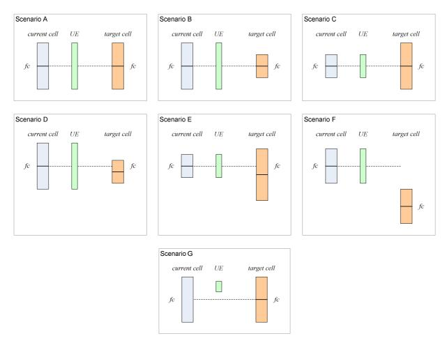
Figure 10.1.3-1: Inter and Intra-frequency measurements scenarios
