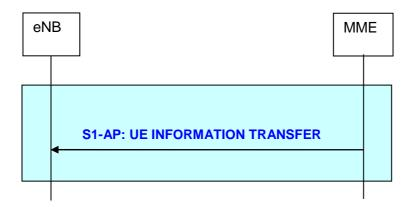
Figure 19.2.2.29: UE Information Transfer procedure
