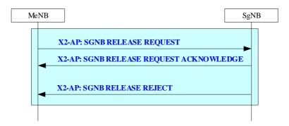
Figure 20.2.2.24-1: MeNB initiated SgNB Release procedure
