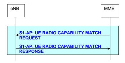
Figure 19.2.2.21-1: UE Radio Capability Match procedure
