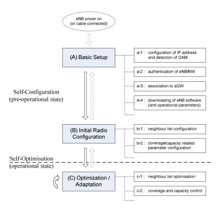
Figure 22.1-1: Ramifications of Self-Configuration /Self-Optimisation functionality
