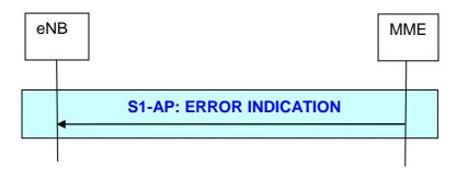
Figure 19.2.2.7.2b-1: MME initiated Error Indication procedure
