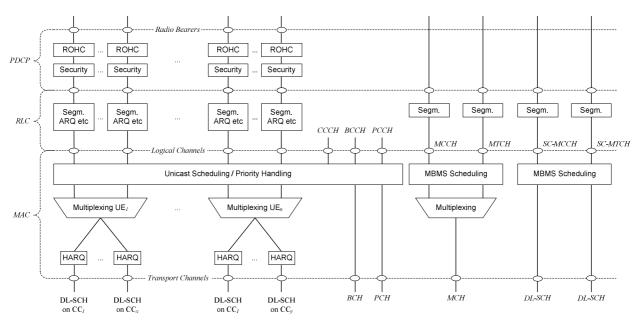
Figure 6.4-1: Layer 2 Structure for DL with CA configured
