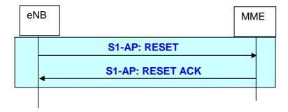
Figure 19.2.2.7.1a-1: eNB initiated Reset procedure
