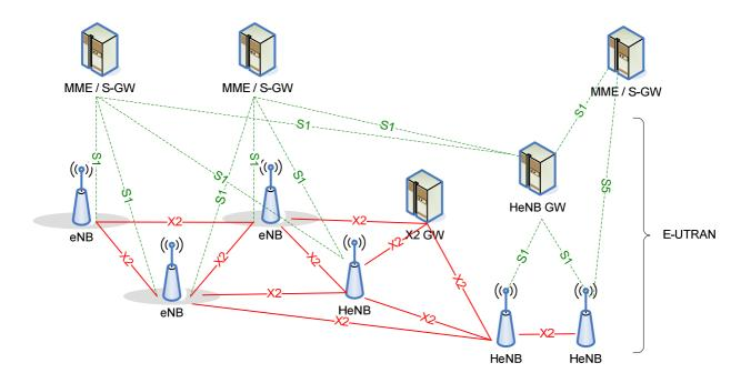
Figure 4.6.1-2: Overall E-UTRAN Architecture with deployed HeNB GW and X2 GW.
