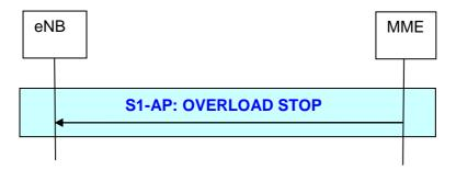
Figure 19.2.2.12.2-1: Overload Stop procedure
