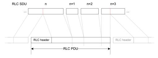
Figure 6.2.2-1: RLC PDU Structure
