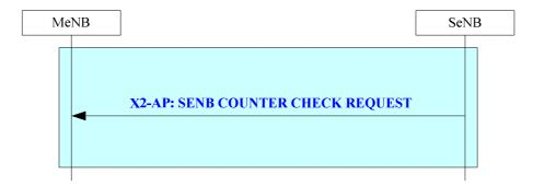
Figure 20.2.2.2g-1: SeNB Counter Check procedure
