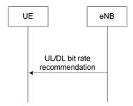
Figure 23.15.1-1: UL or DL bit rate recommendation
