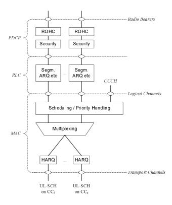
Figure 6.4-2: Layer 2 Structure for UL with CA configured
