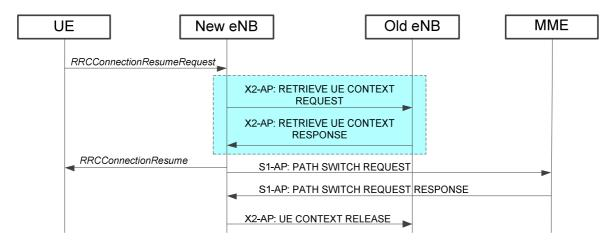
Figure 20.2.2.19-1: Retrieve UE Context procedure (highlighted in blue) for cases of UE context resumption. Successful case
