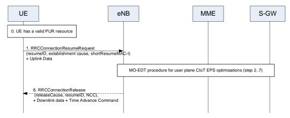
Figure 7.3d-3: Transmission using PUR for the User Plane CloT EPS Optimisation
