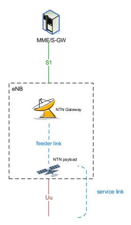
Figure 4.12-1: Overall illustration of an NTN
