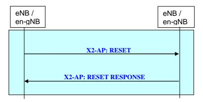
Figure 20.2.2.9-1: Reset procedure between eNBs
