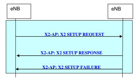
Figure 20.2.2.7-1: X2 Setup procedure
