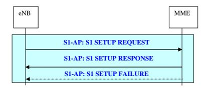
Figure 19.2.2.8-1: S1 Setup procedure
