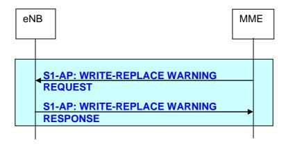
Figure 19.2.2.13.1-1: Write-Replace Warning procedure
