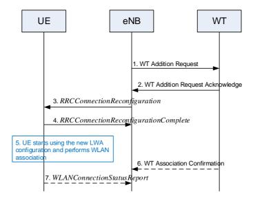
Figure 22A.1.7.1-1: WT Addition procedure
