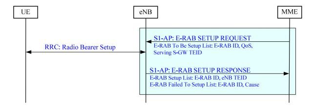
Figure 19.2.2.4.1-1: E-RAB Setup procedure
