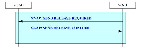
Figure 20.2.2.2f-1: SeNB initiated SeNB Release procedure
