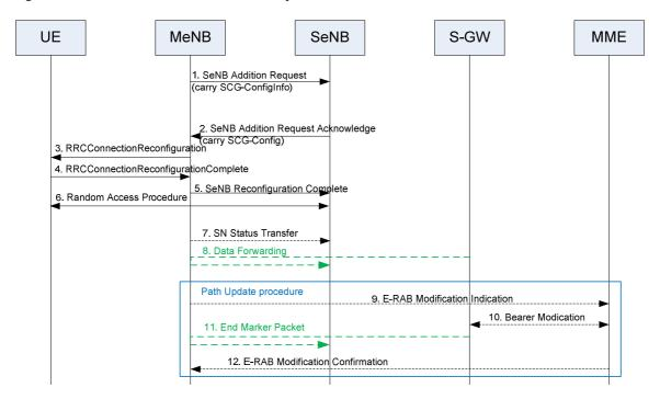
Figure 10.1.2.8.1-1: SeNB Addition procedure
