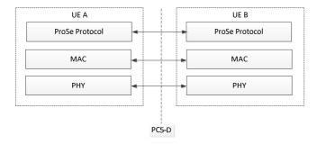
Figure 23.11.1-1: PC5 interface for sidelink discovery (see TS 23.303 [62])
