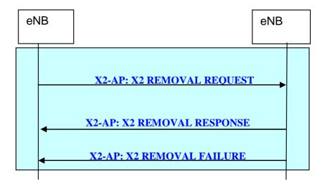
Figure 20.2.2.18-1: X2 Removal procedure
