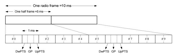
Figure 5.1-2: Frame structure type 2 (for 5ms switch-point periodicity)
