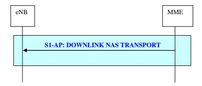
Figure 19.2.2.6-3: Downlink NAS Transport procedure
