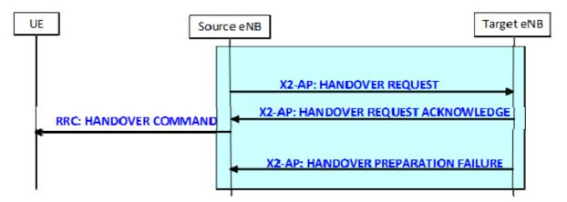
Figure 20.2.2.1-1: Handover Preparation procedure
