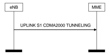
Figure 19.2.2.16.2-1: Uplink S1 CDMA2000 Tunnelling procedure
