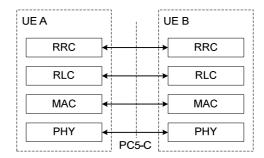
Figure 23.10.2.2-1: Control-Plane protocol stack for SBCCH
