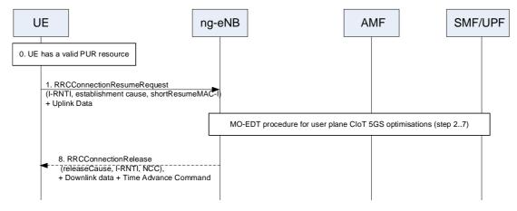
Figure 7.3d-4: Transmission using PUR for the User Plane CloT 5GS Optimisation
