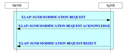
Figure 20.2.2.2-1: MeNB initiated SqNB Modification Preparation procedure
