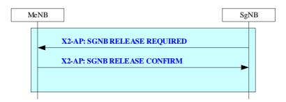
Figure 20.2.2.25-1: SgNB initiated SgNB Release procedure
