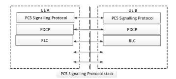
Figure 23.10.2.2-2: Control-Plane protocol stack for one-to-one sidelink communication
