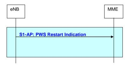
Figure 19.2.2.22-1: PWS Restart Indication procedure
