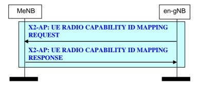
Figure 20.2.2.33-1: UE Radio Capability ID Mapping procedure
