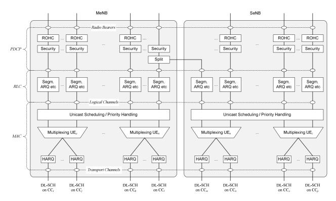
Figure 6.5-1: Layer 2 Structure for DL with CA and DC configured
