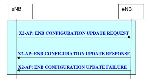
Figure 20.2.2.8-1: eNB Configuration Update procedure
