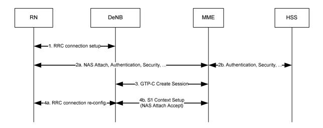
Figure 4.7.6.1-1: RN attach procedure
