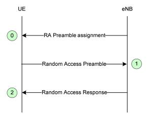
Figure 10.1.5.2-1: Non-contention based Random Access Procedure
