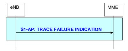
Figure 19.2.2.19.2-1: Trace Failure Indication procedure
