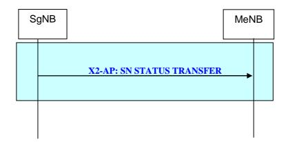
Figure 20.2.2.4-3: SgNB-initiated SN Status Transfer procedure for EN-DC.
