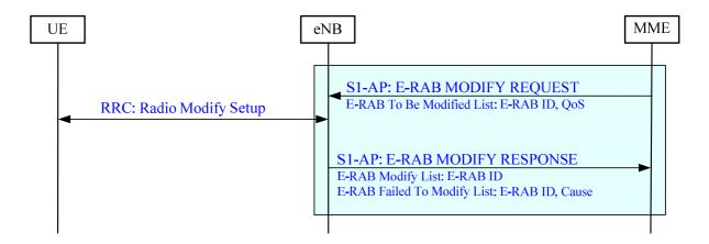
Figure 19.2.2.4.2-1: E-RAB Modification procedure
