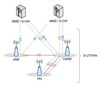
Figure 4.7.2-1: Overall E-UTRAN Architecture supporting RNs
