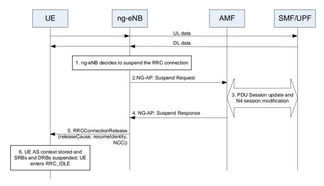
Figure 7.3a.3-1a: RRC Connection Suspend procedure in 5GS
