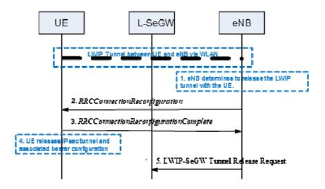
Figure 22A.3.1.3-1: LWIP tunnel release procedure
