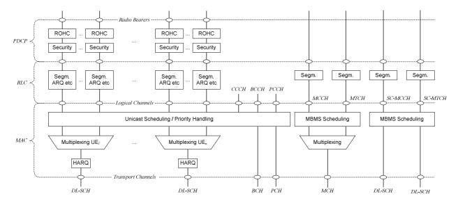
Figure 6-1: Layer 2 Structure for DL
