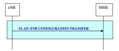
Figure 19.2.2.9a-1: eNB Configuration Transfer procedure
