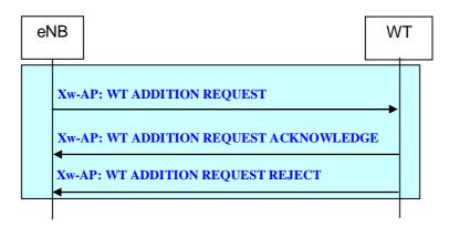
Figure 22B.2.2.1-1: WT Addition Preparation procedure
