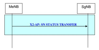
Figure 20.2.2.4-2: MeNB-initiated SN Status Transfer procedure for EN-DC.
