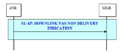
Figure 19.2.2.6-4: Downlink NAS Non Delivery Indication procedure
