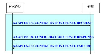
Figure 20.2.2.29-2: EN-DC Configuration Update procedure triggered by the en-gNB.
