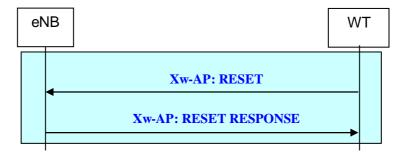
Figure 22B.2.2.12.1-1: Reset procedure initiated by WT
