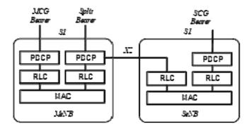
Figure 4.9.2-1: Radio Protocol Architecture for Dual Connectivity
