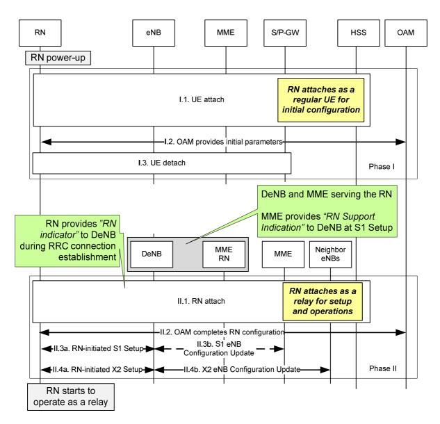
Figure 4.7.6.3-1: RN startup procedure
