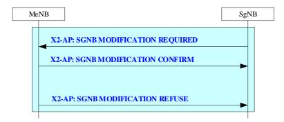
Figure 20.2.2.23-1: SgNB initiated SgNB Modification procedure
