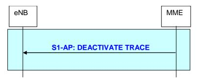
Figure 19.2.2.19.3-1: Deactivate Trace procedure
