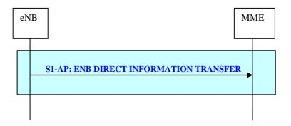
Figure 19.2.2.14-1: eNB Direct Information Transfer procedure
