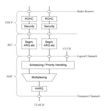
Figure 6-2: Layer 2 Structure for UL
