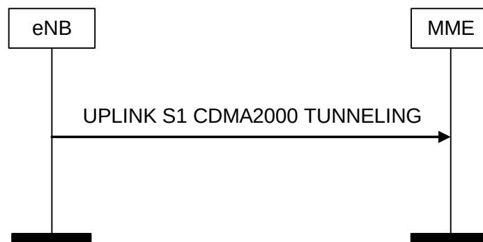
Figure 19.2.2.16.2-1: Uplink S1 CDMA2000 Tunnelling procedure
