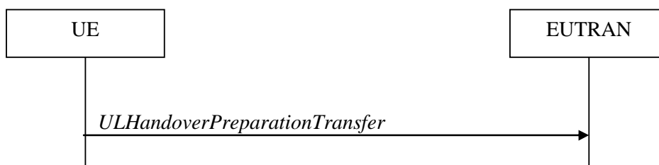
Figure 5.4.5.1-1: UL handover preparation transfer
