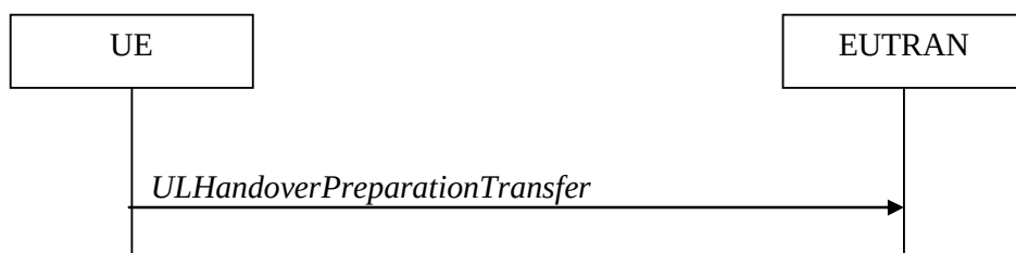
Figure 5.4.5.1-1: UL handover preparation transfer
