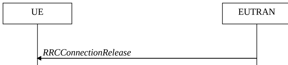
Figure 5.3.8.1-1: RRC connection release, successful
