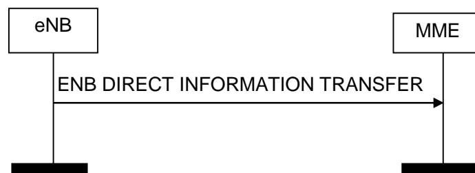
Figure 8.13.1.2-1: ENB Direct Information Transfer procedure. Successful operation.
