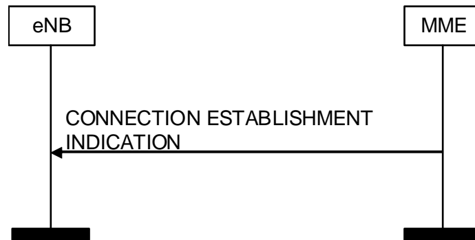
Figure 8.3.9.2-1: Connection Establishment Indication procedure. Successful operation.
