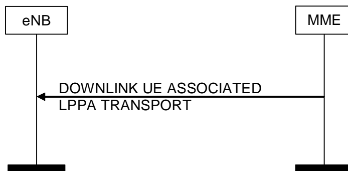
Figure 8.17.2.1-1: DOWNLINK UE ASSOCIATED LPPA Transport Procedure
