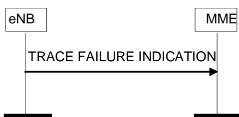
Figure 8.10.2.2-1: Trace Failure Indication procedure.
