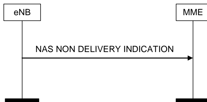
Figure 8.6.2.4-1: NAS NON DELIVERY INDICATION Procedure
