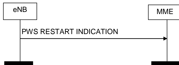
Figure 8.12.3.2-1: PWS Restart Indication procedure. Successful operation.
