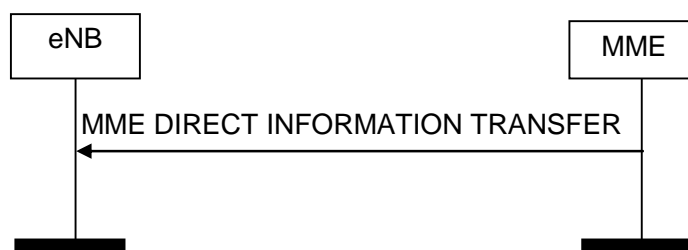
Figure 8.14.1.2-1: MME Direct Information Transfer procedure. Successful operation.
