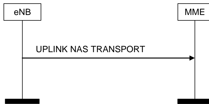
Figure 8.6.2.3-1: UPLINK NAS TRANSPORT Procedure
