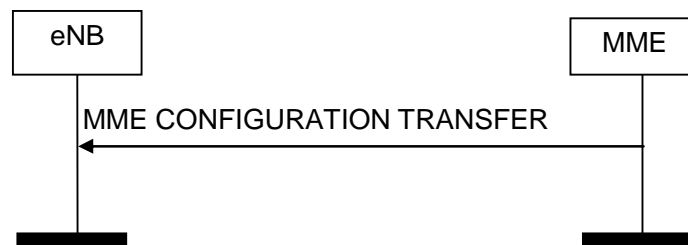
Figure 8.16.2.1-1: MME Configuration Transfer procedure. Successful operation.
