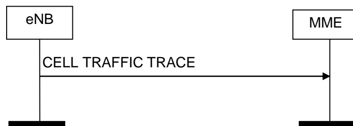
Figure 8.10.4.2-1: Cell Traffic Trace procedure. Successful operation.
