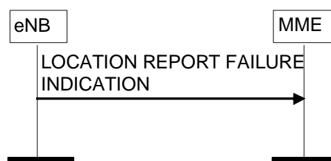
Figure 8.11.2.2-1: Location Report Failure Indication procedure.
