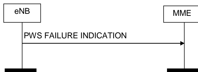
Figure 8.12.4.2-1: PWS Failure Indication procedure. Successful operation.
