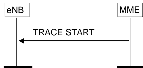
Figure 8.10.1.2-1: Trace Start procedure.
