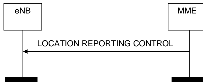
Figure 8.11.1.2-1: Location Reporting Control procedure. Successful operation.
