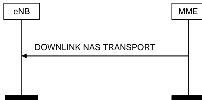
Figure 8.6.2.2-1: DOWNLINK NAS Transport Procedure
