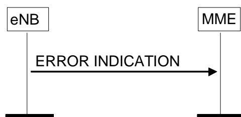
Figure 8.7.2.2-2: Error Indication procedure, eNB originated. Successful operation.
