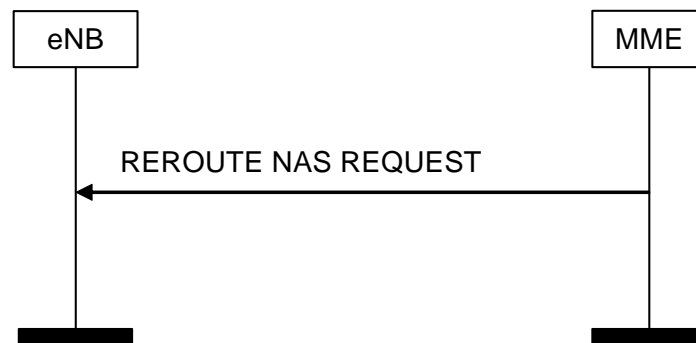
Figure 8.6.2.5-1: Reroute NAS Request Procedure
