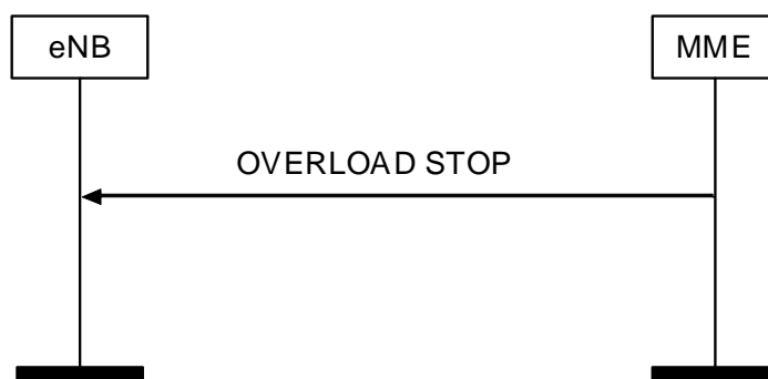
Figure 8.7.7.2.-1: Overload Stop procedure
