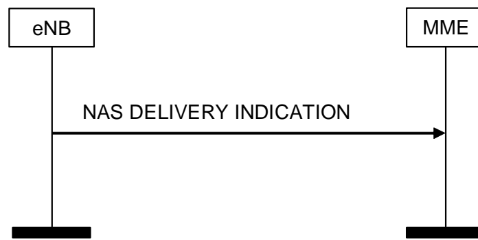
Figure 8.6.2.4a-1: NAS DELIVERY INDICATION Procedure
