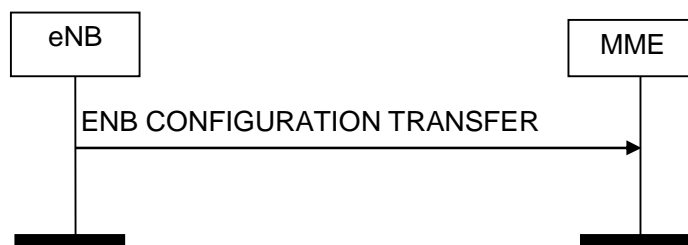
Figure 8.15.2.1-1: eNB Configuration Transfer procedure. Successful operation.
