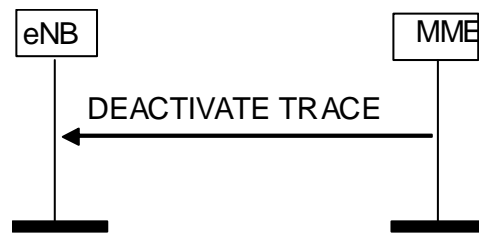
Figure 8.10.3.2-1: Deactivate Trace procedure. Successful operation.
