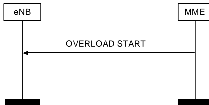
Figure 8.7.6.2-1: Overload Start procedure
