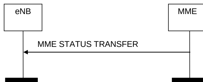
Figure 8.4.7.2-1: MME Status Transfer procedure
