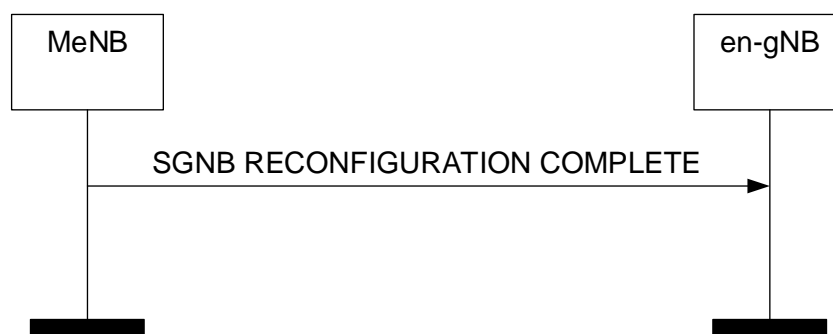
Figure 8.7.5.2-1: SgNB Reconfiguration Complete procedure, successful operation.
