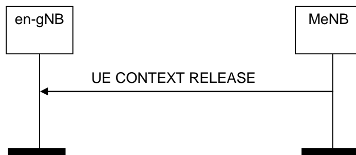
Figure 8.2.3.2-3: UE Context Release, successful operation for EN-DC
