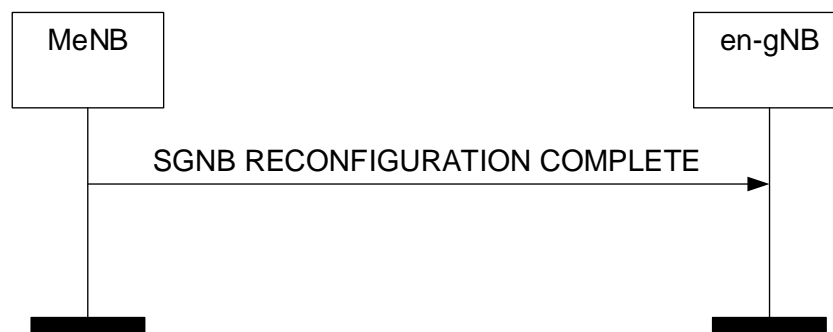
Figure 8.7.5.2-1: SgNB Reconfiguration Complete procedure, successful operation.
