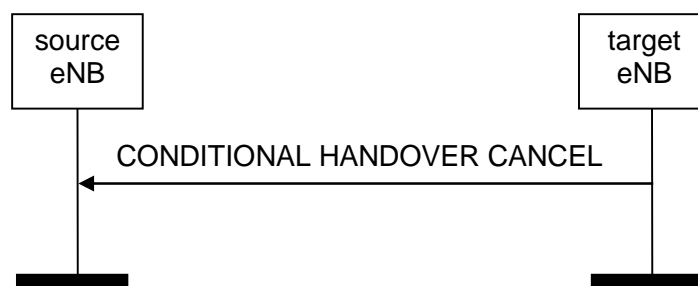
Figure 8.2.6.2-1: Conditional Handover Cancel, successful operation
