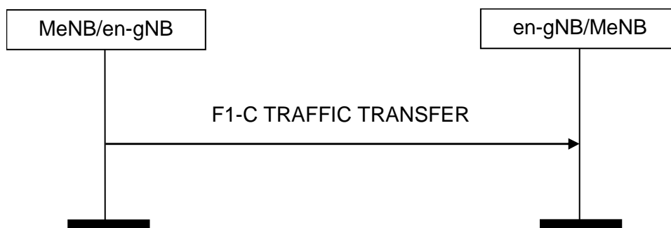
Figure 8.8.1.2-1: F1-C Traffic Transfer procedure, successful operation.
