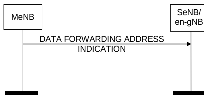
Figure 8.3.15.2-2: Data Forwarding Address Indication for Conditional Handover, successful operation
