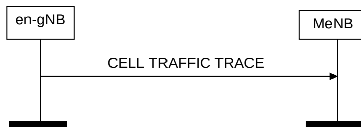
Figure 8.7.23.2-1: Cell Traffic Trace procedure. Successful operation.
