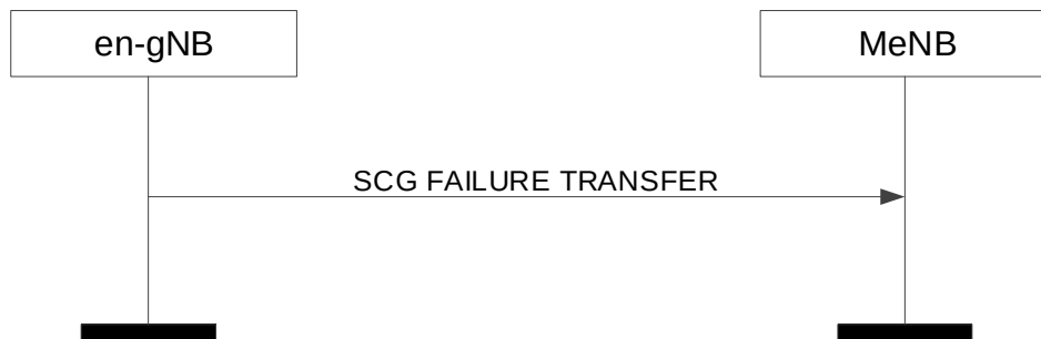
Figure 8.7.27.2-1: SCG Failure Transfer, successful operation
