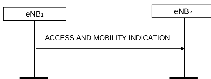
Figure 8.3.16.2-2: Access and Mobility Indication. Successful operation – eNB-initiated
