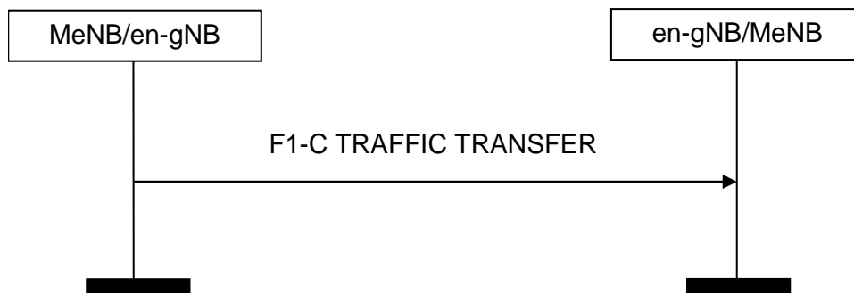
Figure 8.8.1.2-1: F1-C Traffic Transfer procedure, successful operation.
