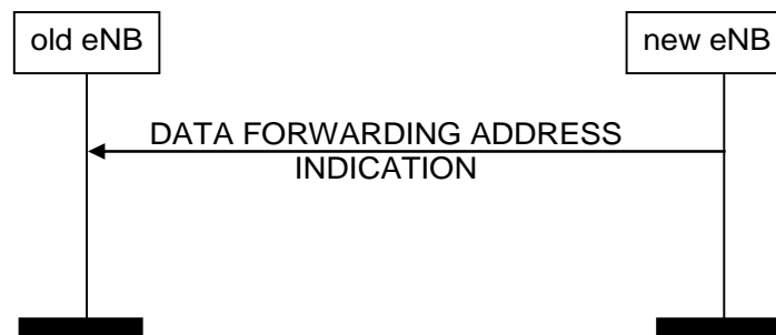
Figure 8.3.15.2-1: Data Forwarding Address Indication, successful operation
