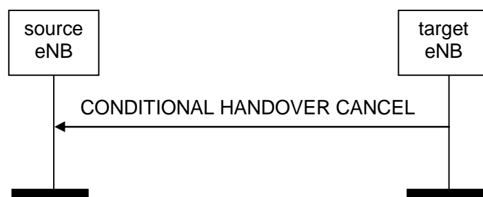
Figure 8.2.6.2-1: Conditional Handover Cancel, successful operation
