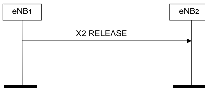
Figure 8.4.2-1: X2AP Release, successful operation
