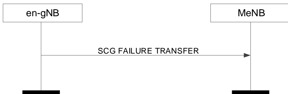
Figure 8.7.27.2-1: SCG Failure Transfer, successful operation
