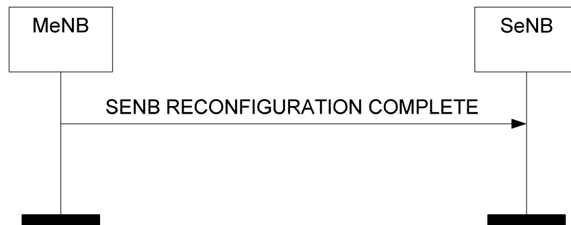
Figure 8.6.2.2-1: SeNB Reconfiguration Complete procedure, successful operation.
