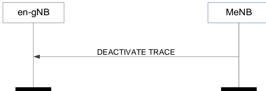
Figure 8.7.20.2-1: Deactivate Trace, successful operation
