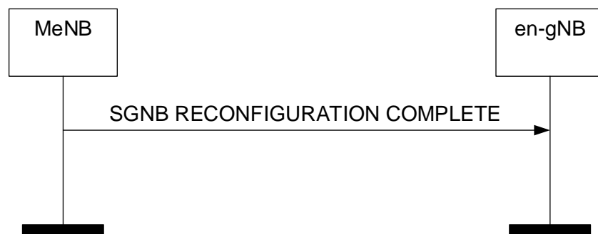
Figure 8.7.5.2-1: SgNB Reconfiguration Complete procedure, successful operation.
