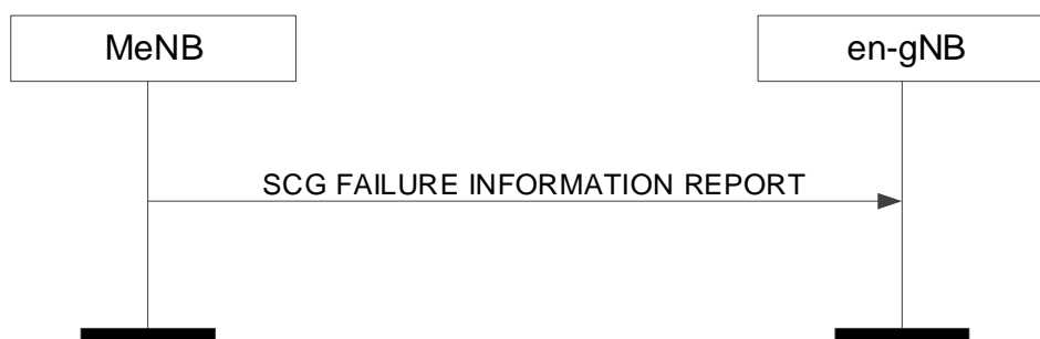
Figure 8.7.26.2-1: SCG Failure Information Report, successful operation
