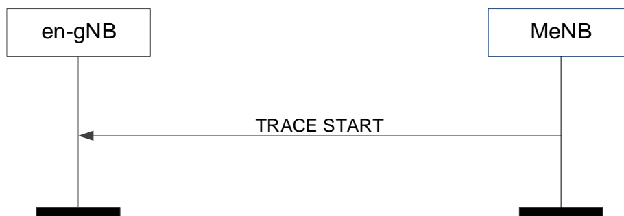
Figure 8.7.19.2-1: Trace Start, successful operation
