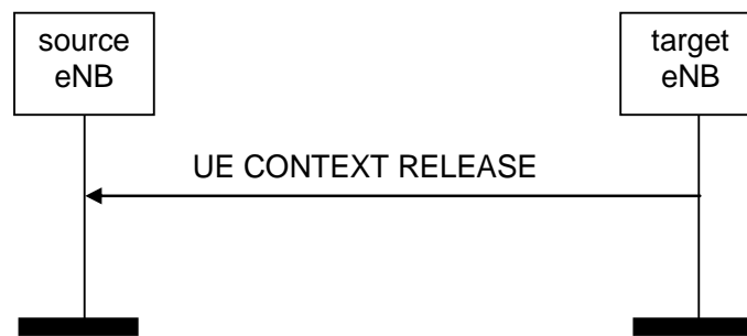
Figure 8.2.3.2-1: UE Context Release, successful operation for handover
