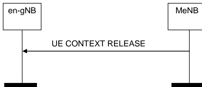
Figure 8.2.3.2-3: UE Context Release, successful operation for EN-DC
