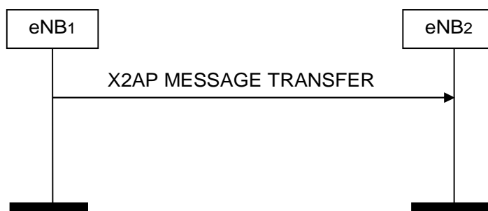
Figure 8.5.2-1: X2AP Message Transfer, successful operation
