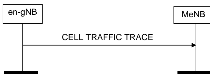
Figure 8.7.23.2-1: Cell Traffic Trace procedure. Successful operation.
