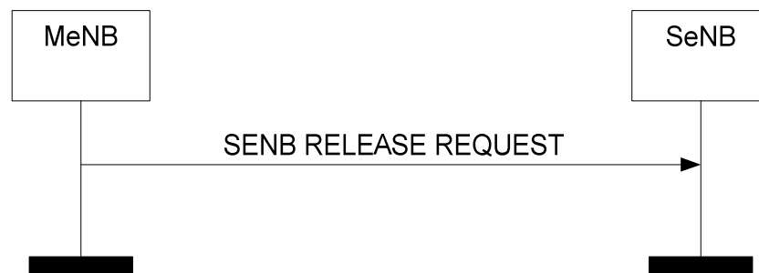
Figure 8.6.5.2-1: MeNB initiated SeNB Release, successful operation
