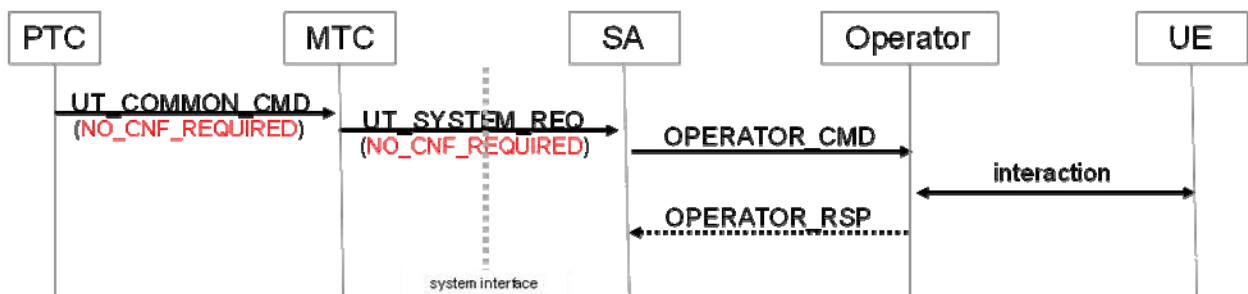
Figure E.1-2: No confirmation (manual intervention)
