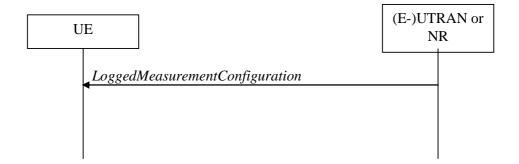
Figure 5.1.1.1-1: MDT measurement configuration for Logged MDT
