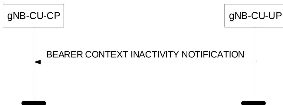
Figure 8.3.6.2-1: Bearer Context Inactivity Notification procedure: Successful Operation.
