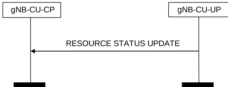
Figure 8.2.10.2-1: Resource Status Reporting, successful operation
