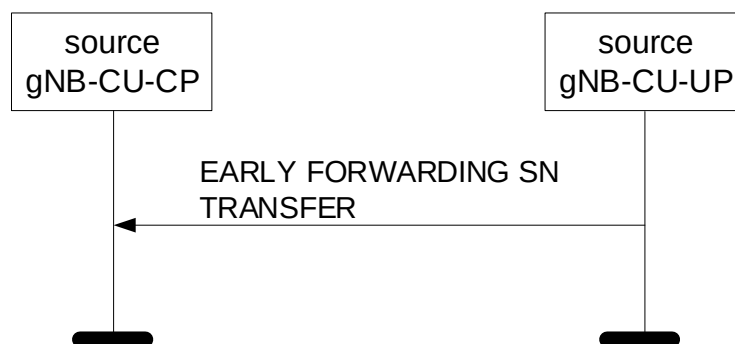
Figure 8.3.12.2-1: Early Forwarding SN Transfer procedure: Successful Operation.
