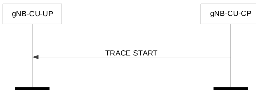
Figure 8.4.1.2-1: Trace start procedure: Successful Operation.
