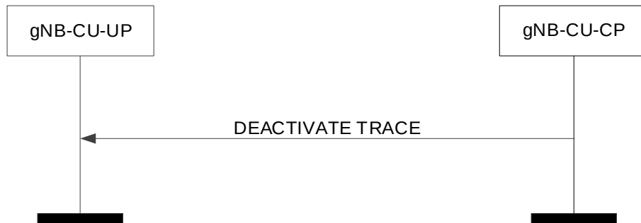
Figure 8.4.2.2-1: Deactivate trace procedure: Successful Operation.
