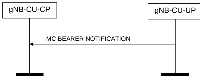
Figure 8.6.2.6.2-1: MC Bearer Notification procedure: Successful Operation.
