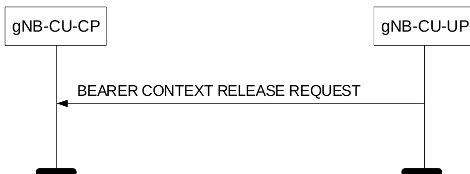
Figure 8.3.5.2-1: Bearer Context Release Request procedure: Successful Operation.
