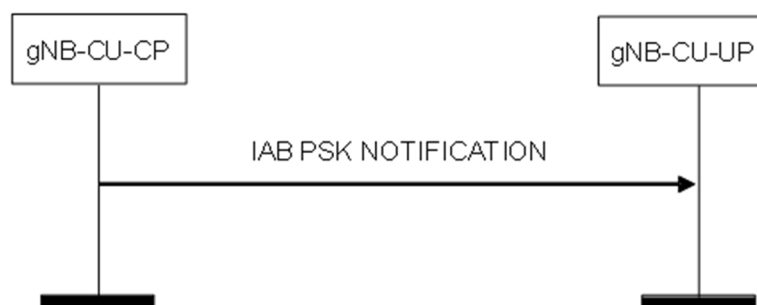
Figure 8.5.2.2-1: IAB PSK Notification procedure: Successful Operation.
