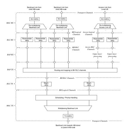
Figure 6.1-5: UL L2-structure at IAB-node
