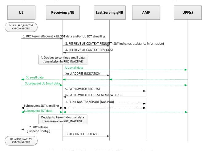
Figure 18.2-1. RA-based SDT with UE context relocation
