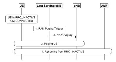
Figure 9.2.2.4.2-1: Network triggered transition from RRC\_INACTIVE to RRC\_CONNECTED
