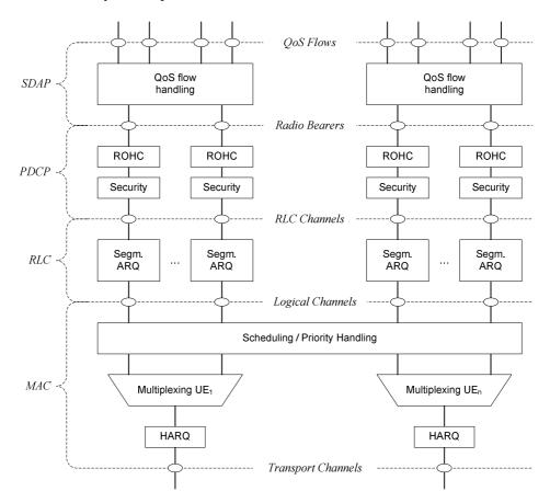
Figure 6.1-1: Downlink Layer 2 Structure
