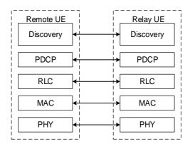
Figure 16.12.3-1: Protocol Stack of Discovery Message for UE-to-Network Relay
