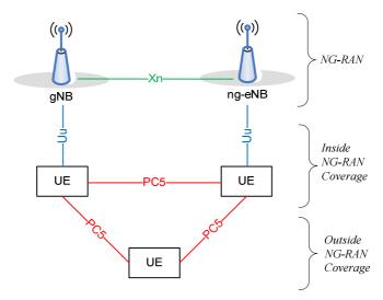
Figure 16.9.1-1: NG-RAN Architecture supporting the PC5 interface
