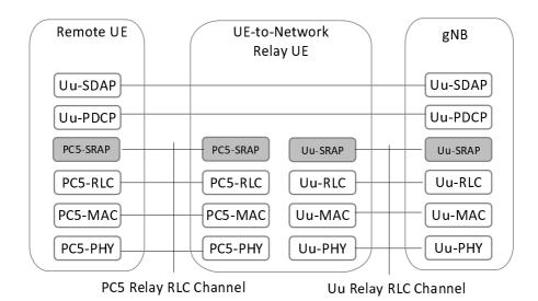
Figure 16.12.2.1-1: User plane protocol stack for L2 UE-to-Network Relay
