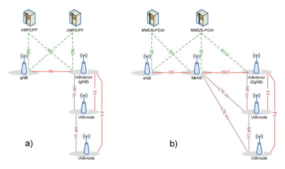
Figure 4.7.1-1: IAB architecture; a) IAB-node using SA mode with 5GC; b) IAB-node using EN-DC
