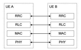
Figure 16.9.2.1-3: Control plane protocol stack for SBCCH.
