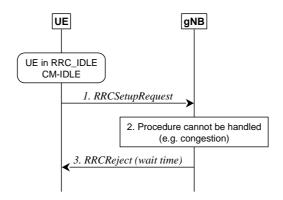
Figure 9.2.1.3-2: Rejection of UE triggered transition from RRC\_IDLE
