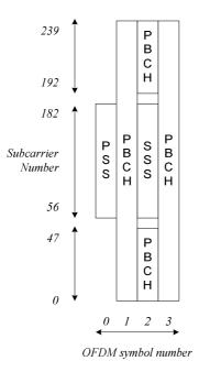
Figure 5.2.4-1: Time-frequency structure of SSB
