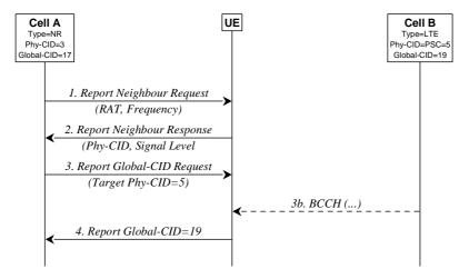
Figure 15.3.3.5-1: Automatic Neighbour Relation Function in case of E-UTRAN detected cell
