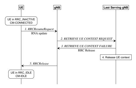
Figure 9.2.2.5-3: RNA update procedure with transition to RRC\_IDLE
