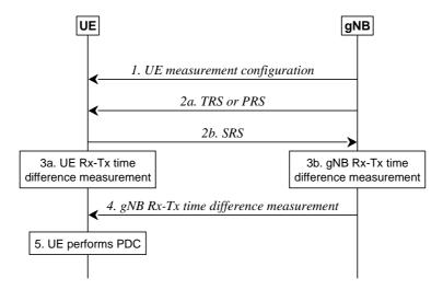
Figure 16.8-1: Signalling Procedure of UE-side RTT-based PDC
