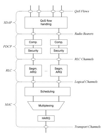
Figure 6.1-2: Uplink Layer 2 Structure
