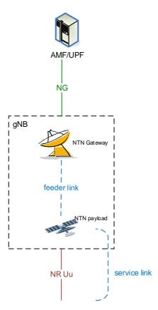
Figure 16.14.1-1: Overall illustration of an NTN
