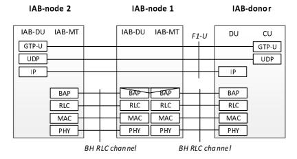
Fig. 4.7.2-1: Protocol stack for the support of F1-U protocol
