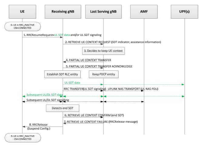
Figure 18.3-1. RA-based SDT without UE context relocation
