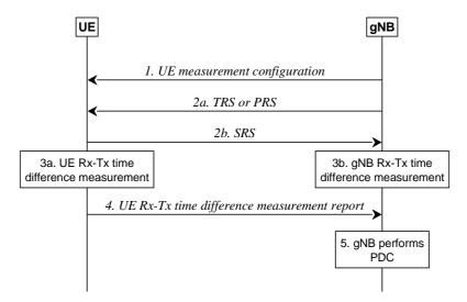
Figure 16.8-2: Signalling Procedure of gNB-side RTT-based PDC
