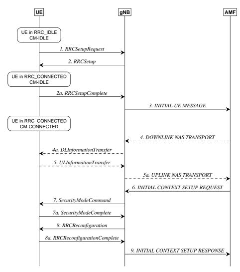
Figure 9.2.1.3-1: UE triggered transition from RRC\_IDLE to RRC\_CONNECTED
