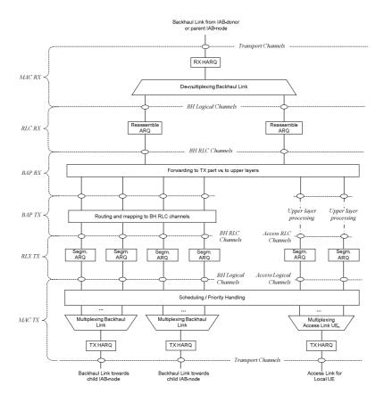
Figure 6.1-4: DL L2-structure at IAB-node
