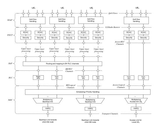
Figure 6.1-3: DL L2-structure for user plane at IAB-donor
