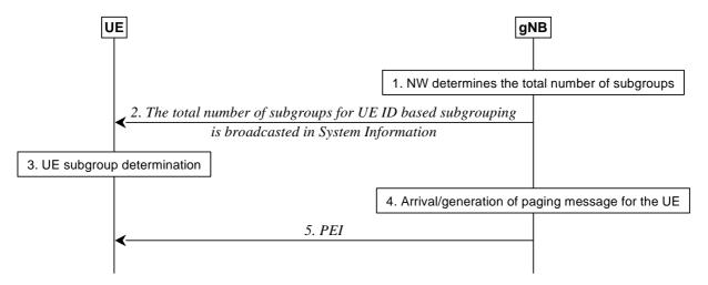
Figure 9.2.5-2: Procedure for UE ID based subgrouping
