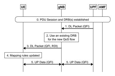
Figure A.2-1: DL data with new QFI sent over existing DRB
