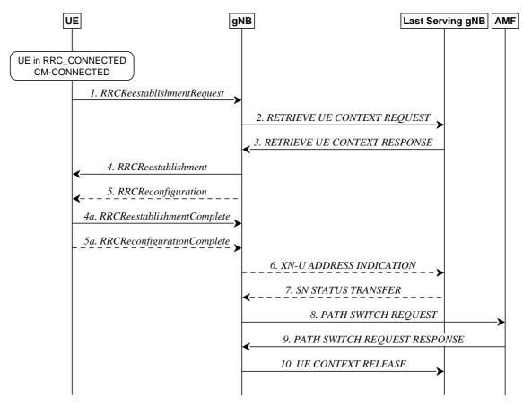
Figure 9.2.3.3-1: Re-establishment procedure
