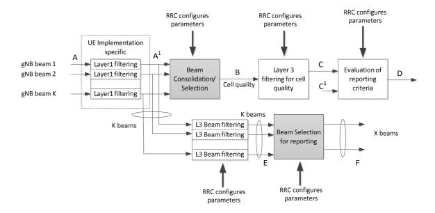
Figure 9.2.4-1: Measurement Model
