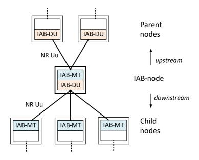
Figure 4.7.1-2: Parent- and child-node relationship for IAB-node
