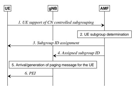
Figure 9.2.5-1: Procedure for CN controlled subgrouping
