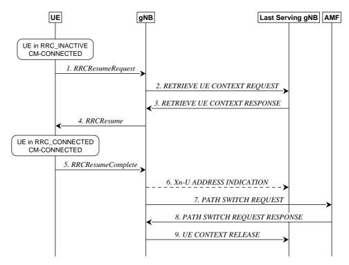
Figure 9.2.2.4.1-1: UE triggered transition from RRC\_INACTIVE to RRC\_CONNECTED (UE context retrieval success)
