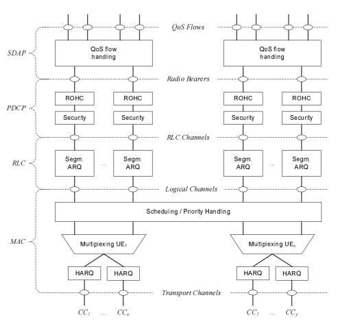
Figure 6.7-1: Layer 2 Structure for DL with CA configured
