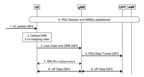
Figure A.6-1: UL packet with a new QoS flow for which a mapping does not exist in UE
