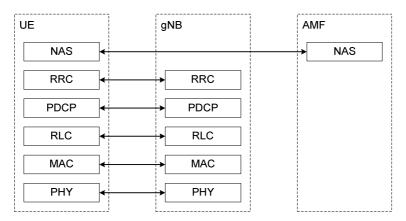
Figure 4.4.2-1: Control Plane Protocol Stack
