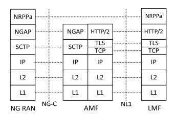
Figure 6.5.1-1: Protocol Layering for LMF to NG-RAN Signalling
