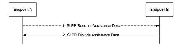
Figure 8.15.4.2.2-1: Assistance Data transfer procedure.
