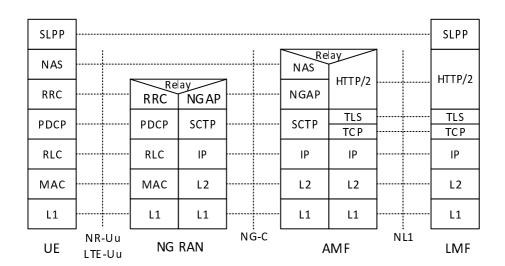
Figure 6.4.1-2: Protocol Layering for LMF to UE SLPP Signalling
