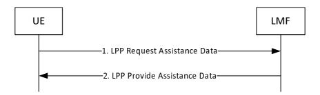
Figure 8.4.3.2.2-1: UE-initiated Assistance Data Transfer Procedure
