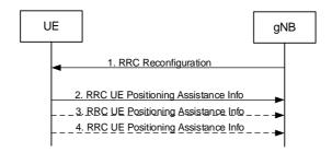
Figure 7.4.1.2-1: RRC procedure for UE TxTEG
