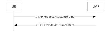
Figure 8.1.3.2.2-1: UE-initiated Assistance Data Transfer Procedure
