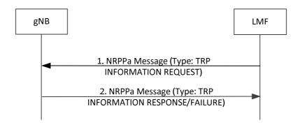
Figure 8.13.3.2.1-2: LMF-initiated TRP Information Exchange Procedure
