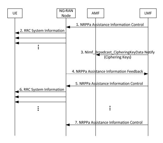
Figure 7.5.2-1: Procedures to support broadcast of assistance data.
