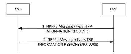
Figure 8.14.3.2.1-2: LMF-initiated TRP Information Exchange Procedure
