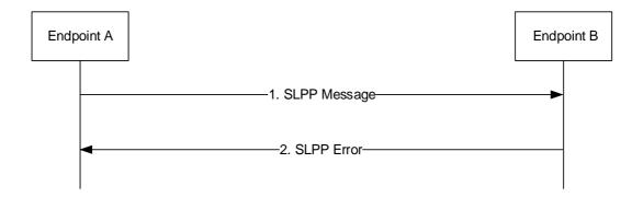
Figure 7.11.2.4-1: SLPP Error handling
