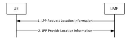
Figure 8.12.3.1.3.1-1: LMF-initiated Location Information Transfer Procedure
