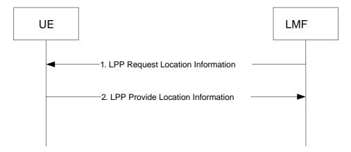
Figure 8.8.3.2-1: LMF-initiated Location Information Transfer Procedure
