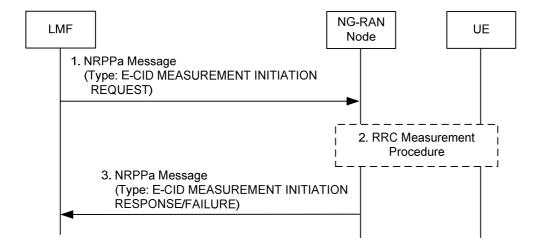
Figure 8.3.4.3.1-1: LMF-initiated Position Measurement Procedure
