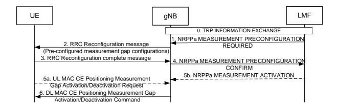
Figure 7.7.2-1: Pre-configured measurement gap configuration and activation procedure
