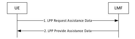
Figure 8.2.3.2.1.2-1: UE-initiated Assistance Data Transfer Procedure
