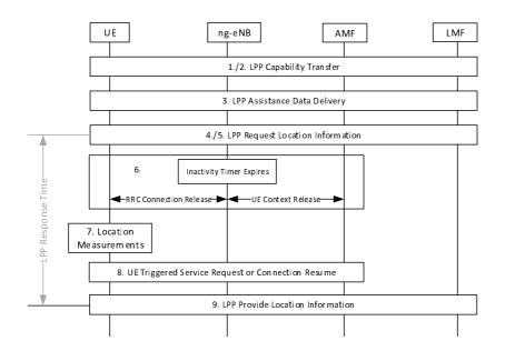
Figure 7.1.3-1: UE positioning measurements in RRC\_IDLE state.
