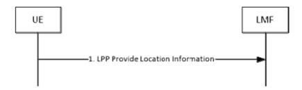
Figure 8.10.3.1.3.2-1: UE-initiated Location Information Delivery Procedure.
