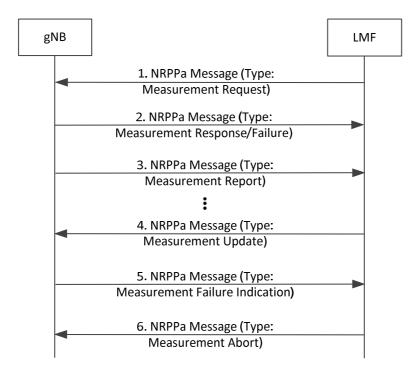
Figure 8.14.3.3-1: LMF-initiated Location Information Transfer Procedure
