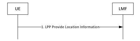
Figure 8.4.3.3.2-1: UE-initiated Location Information Delivery Procedure
