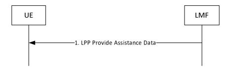
Figure 8.1.3.2.1-1: LMF-initiated Assistance Data Delivery Procedure
