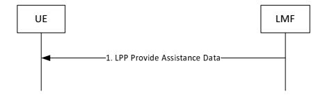
Figure 8.7.3.2.1-1: LMF-initiated Assistance Data Delivery Procedure
