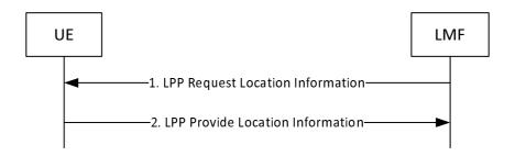
Figure 8.4.3.3.1-1: LMF-initiated Location Information Transfer Procedure
