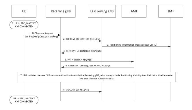
Figure 7.14.3-1: Area-specific SRS Configuration Update Procedure
