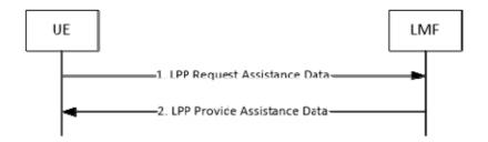
Figure 8.6.3.2.2-1: UE-initiated Assistance Data Transfer Procedure
