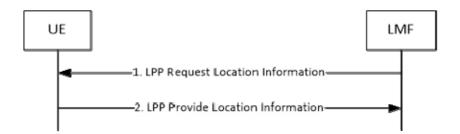
Figure 8.11.3.1.3.1-1: LMF-initiated Location Information Transfer Procedure
