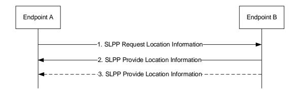
Figure 7.11.2.3-1: SLPP Location Information Transfer procedure
