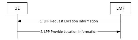
Figure 8.5.3.3.1-1: LMF-initiated Location Information Transfer Procedure
