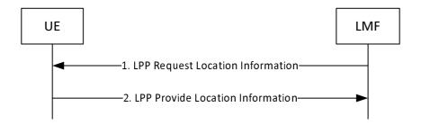
Figure 8.1.3.3.1-1: LMF-initiated Location Information Transfer Procedure
