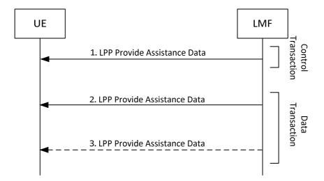
Figure 8.1.3.2.1a-1: LPP Periodic Assistance data delivery procedure
