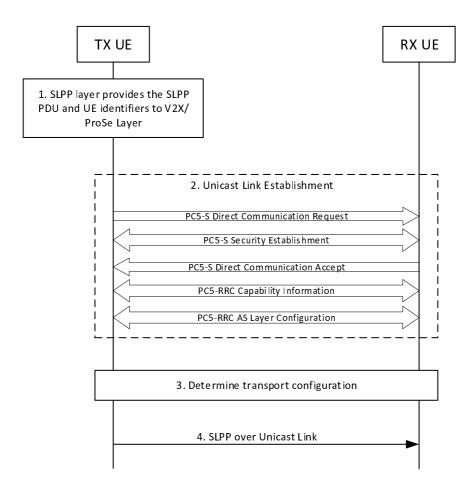
Figure 6.7.2-1: SLPP PDU transfer between UEs
