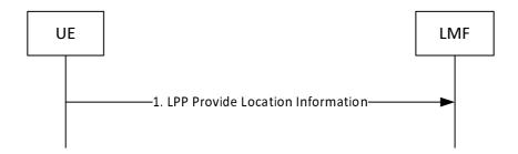
Figure 8.6.3.3.2-1: UE-initiated Location Information Delivery Procedure
