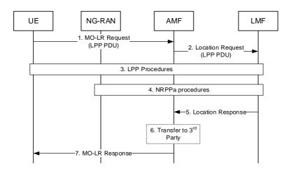
Figure 7.3.3-1: UE Positioning Operations to support an MO-LR
