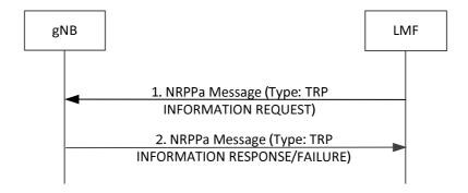
Figure 8.10.3.2.1-1: LMF-initiated TRP Information Exchange Procedure
