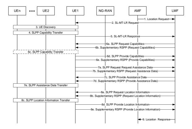
Figure 7.3A.2-1: UE Positioning Operations to support an SL-MT-LR
