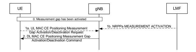
Figure 7.7.2-2: Pre-configured measurement gap deactivation procedure
