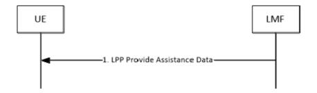
Figure 8.11.3.1.2.1-1: LMF-initiated Assistance Data Delivery Procedure
