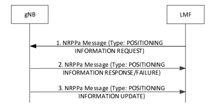
Figure 8.13.3.2.1-1: LMF-initiated UL Information Request Procedure
