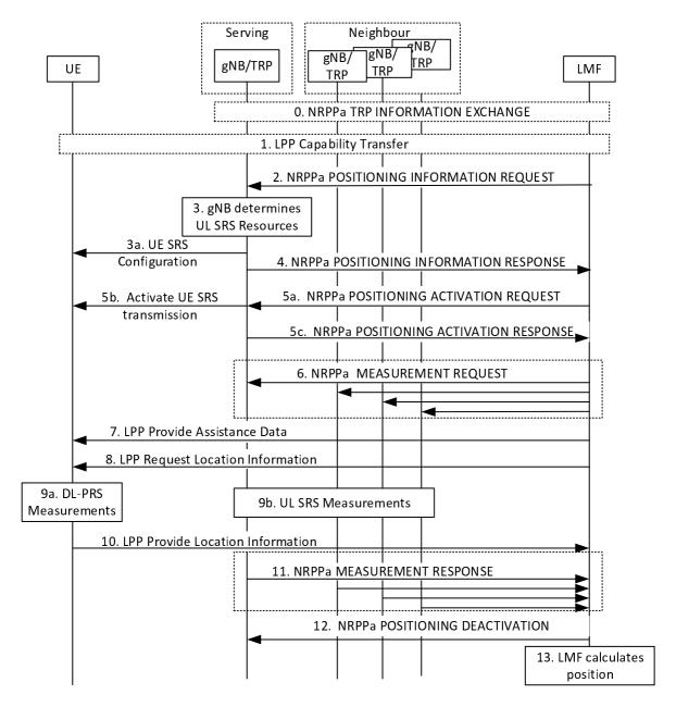
Figure 8.10.4-1: Multi-RTT positioning procedure
