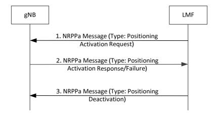
Figure 8.10.3.2.3-1: Positioning Activation/Deactivation Procedure.
