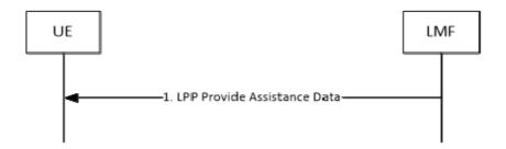
Figure 8.12.3.1.2.1-1: LMF-initiated Assistance Data Delivery Procedure
