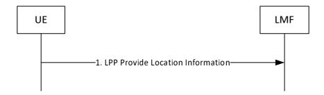
Figure 8.1.3.3.2-1: UE-initiated Location Information Delivery Procedure
