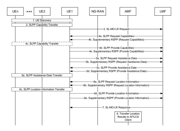
Figure 7.3A.4-1: UE Positioning Operations to support an SL-MO-LR
