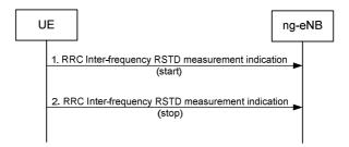
Figure 7.4.2.1-1: Inter-frequency RSTD measurement indication procedure
