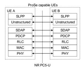
Figure 6.7.1-1: Protocol Layering for UE-to-UE Signalling
