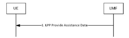
Figure 8.10.3.1.2.1.1-1: LMF-initiated Assistance Data Delivery Procedure
