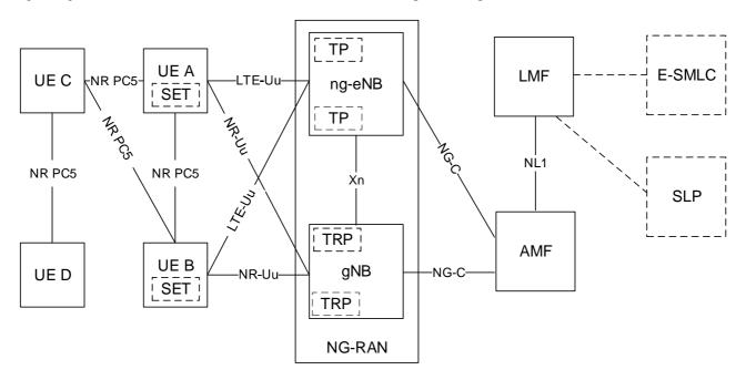
Figure 5.1-1: UE Positioning Overall Architecture applicable to NG-RAN
