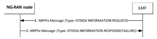
Figure 8.2.3.2.2.1-1: LMF-initiated Assistance Data Delivery Procedure
