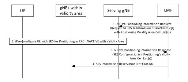
Figure 7.14.2-1: Area-specific SRS (Pre-)configuration Allocation Procedure
