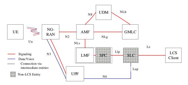
Figure A.2-1: System reference architecture reference for Location Services in reference point representation
