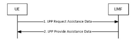
Figure 8.11.3.1.2.2-1: UE-initiated Assistance Data Transfer Procedure
