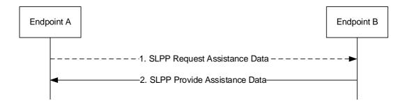
Figure 8.15.5.2.2-1: Assistance Data transfer procedure.
