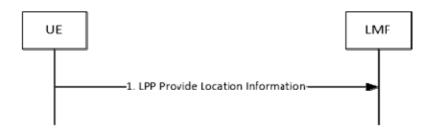
Figure 8.12.3.1.3.2-1: UE-initiated Location Information Delivery Procedure.
