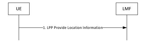
Figure 8.3.3.3.2-1: UE-initiated Location Information Delivery Procedure.
