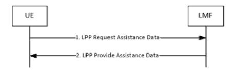
Figure 8.10.3.1.2.1.2-1: UE-initiated Assistance Data Transfer Procedure
