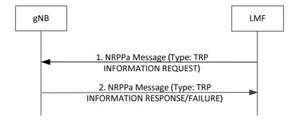
Figure 8.11.3.2.1.1-1: LMF-initiated TRP Information Exchange Procedure
