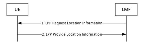
Figure 8.2.3.3.1-1: LMF-initiated Location Information Transfer Procedure
