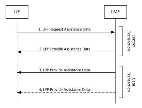
Figure 8.1.3.2.2a-1: UE-initiated Periodic Assistance Data Transfer Procedure
