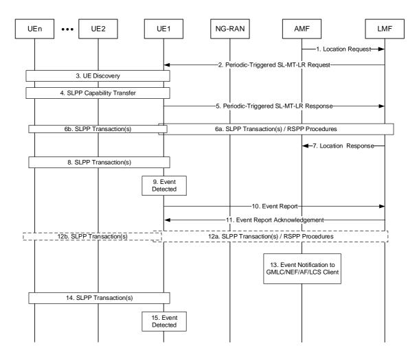
Figure 7.3A.3-1: UE Positioning Operations to support an SL-MT-LR for periodic, triggered Location Events
