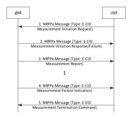
Figure 8.9.4.3-1: LMF-initiated Location Information Transfer Procedure
