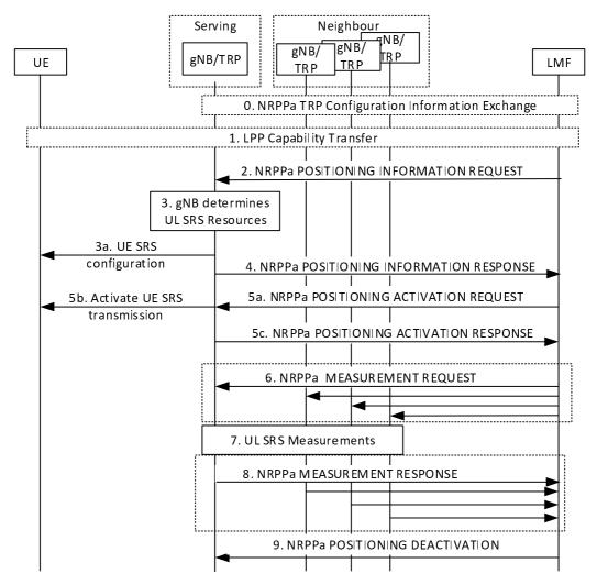
Figure 8.14.3.4-1: UL-AoA positioning procedure
