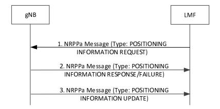
Figure 8.14.3.2.1-1: LMF-initiated UL Information Request Procedure
