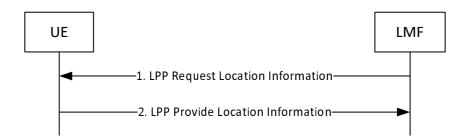
Figure 8.6.3.3.1-1: LMF-initiated Location Information Transfer Procedure
