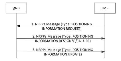
Figure 8.10.3.2.1-2: LMF-initiated UL Information Request Procedure
