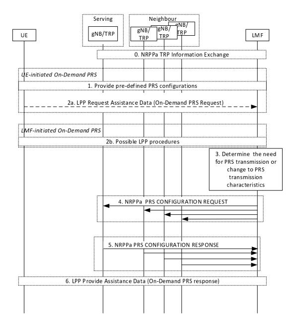
Figure 7.6.2-1: On-Demand PRS transmission procedure
