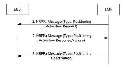
Figure 8.13.3.3a-1: Positioning Activation/Deactivation Procedure.
