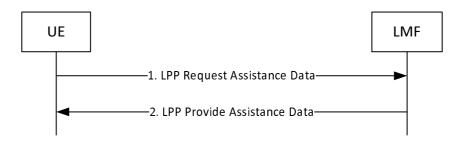
Figure 8.7.3.2.2-1: UE-initiated Assistance Data Transfer Procedure
