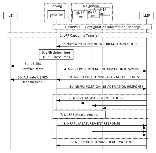
Figure 8.13.3.4-1: UL-TDOA positioning procedure
