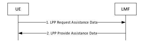
Figure 8.5.3.2.2-1: UE-initiated Assistance Data Transfer Procedure
