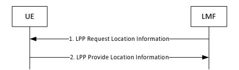
Figure 8.3.3.3-1: LMF-initiated Location Information Transfer Procedure.
