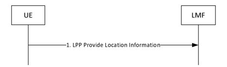
Figure 8.5.3.3.2-1: UE-initiated Location Information Delivery Procedure
