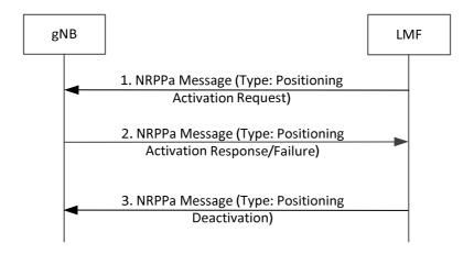
Figure 8.14.3.3a-1: Positioning Activation/Deactivation Procedure.
