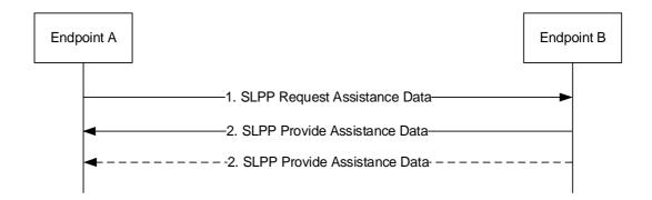
Figure 7.11.2.2-1: SLPP Assistance Data Transfer procedure
