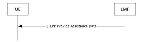
Figure 8.4.3.2.1-1: LMF-initiated Assistance Data Delivery Procedure
