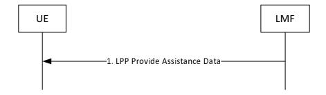
Figure 8.2.3.2.1.1-1: LMF-initiated Assistance Data Delivery Procedure
