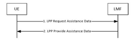
Figure 8.12.3.1.2.2-1: UE-initiated Assistance Data Transfer Procedure
