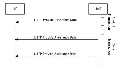
Figure 8.12.3.1.2.1a-1: LPP Periodic Assistance data delivery procedure
