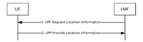
Figure 8.10.3.1.3.1-1: LMF-initiated Location Information Transfer Procedure
