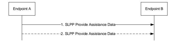
Figure 7.11.2.2-2: SLPP Assistance Data Delivery procedure
