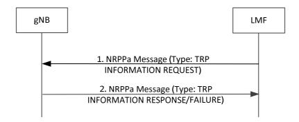
Figure 8.12.3.2.1.1-1: LMF-initiated TRP Information Exchange Procedure
