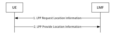
Figure 8.7.3.3.1-1: LMF-initiated Location Information Transfer Procedure
