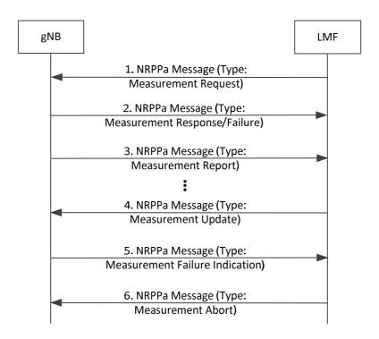
Figure 8.10.3.2.2-1: LMF-initiated Location Information Transfer Procedure
