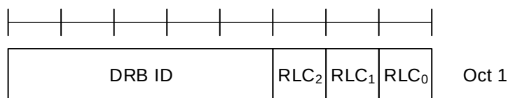
Figure 6.1.3.32-1: Duplication RLC Activation/Deactivation MAC CE
