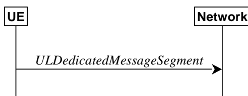
Figure 5.7.7.1-1: UL message segment transfer
