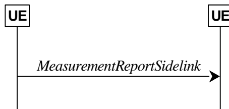
Figure 5.8.10.5.1-1: NR sidelink measurement reporting
