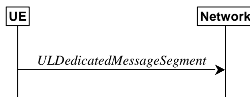
Figure 5.7.7.1-1: UL message segment transfer
