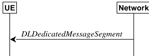
Figure 5.7.6.1-1: DL message segment transfer
