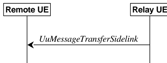
Figure 5.8.9.9.1-1: Uu message transfer in sidelink
