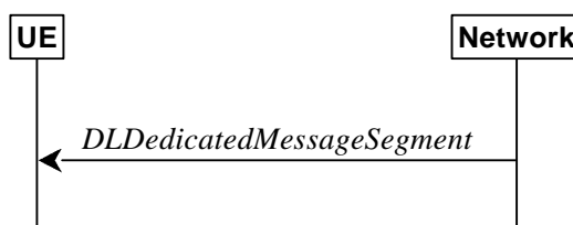
Figure 5.7.6.1-1: DL message segment transfer
