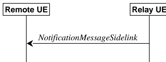
Figure 5.8.9.8.1-1: Notification message in sidelink
