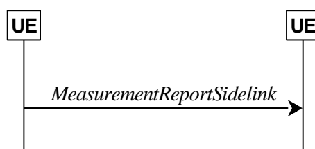
Figure 5.8.10.5.1-1: NR sidelink measurement reporting
