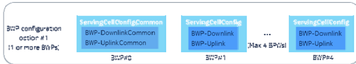
Figure B2-1: BWP#0 configuration without dedicated configuration
