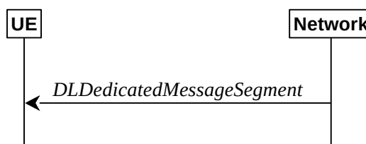
Figure 5.7.6.1-1: DL message segment transfer
