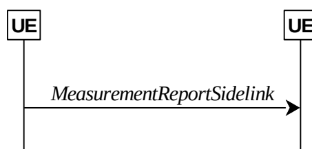
Figure 5.8.10.5.1-1: NR sidelink measurement reporting
