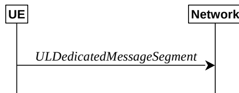
Figure 5.7.7.1-1: UL message segment transfer
