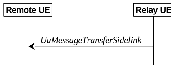
Figure 5.8.9.9.1-1: Uu message transfer in sidelink
