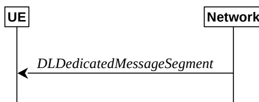
Figure 5.7.6.1-1: DL message segment transfer
