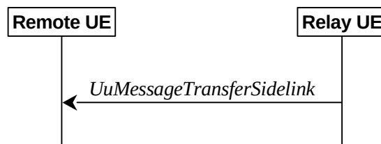
Figure 5.8.9.9.1-1: Uu message transfer in sidelink
