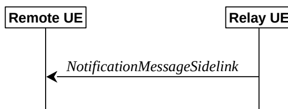
Figure 5.8.9.8.1-1: Notification message in sidelink
