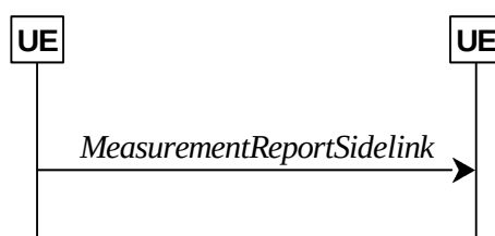
Figure 5.8.10.5.1-1: NR sidelink measurement reporting
