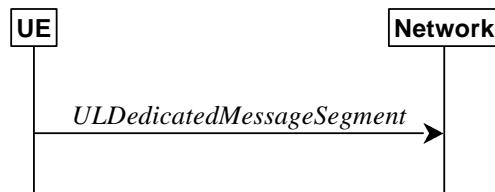
Figure 5.7.7.1-1: UL message segment transfer
