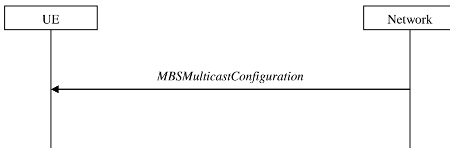
Figure 5.10.2.1-1: Multicast MCCH information acquisition
