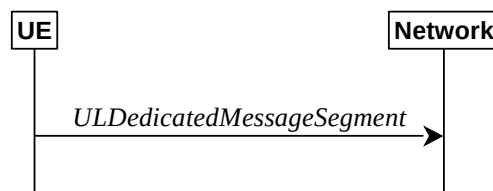
Figure 5.7.7.1-1: UL message segment transfer
