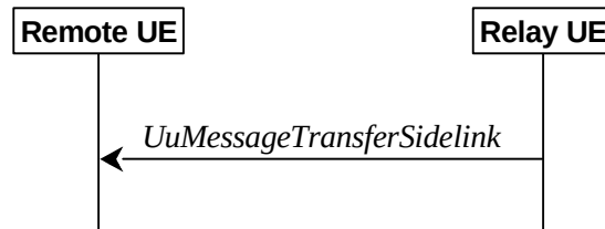
Figure 5.8.9.9.1-1: Uu message transfer in sidelink
