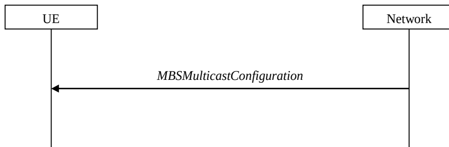
Figure 5.10.2.1-1: Multicast MCCH information acquisition
