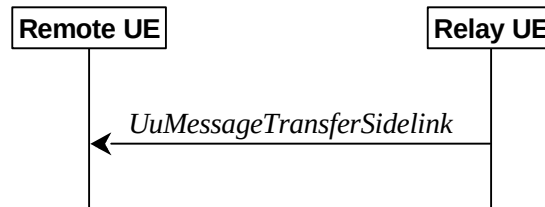
Figure 5.8.9.9.1-1: Uu message transfer in sidelink
