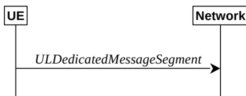
Figure 5.7.7.1-1: UL message segment transfer
