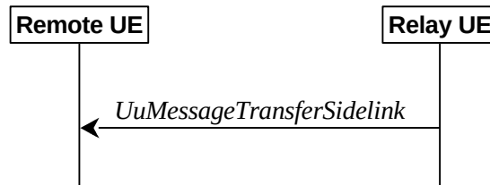
Figure 5.8.9.9.1-1: Uu message transfer in sidelink
