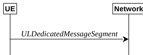
Figure 5.7.7.1-1: UL message segment transfer
