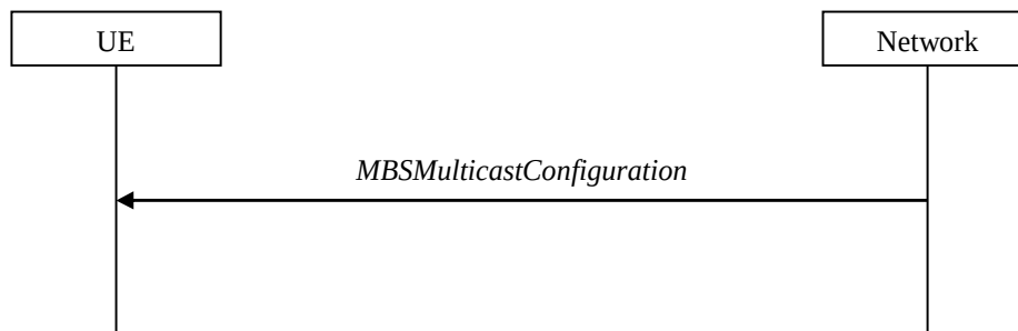
Figure 5.10.2.1-1: Multicast MCCH information acquisition
