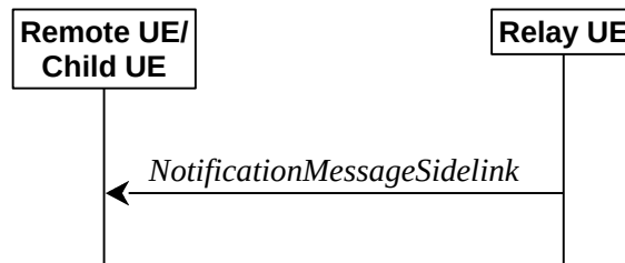
Figure 5.8.9.10.1-1: Notification message in sidelink
