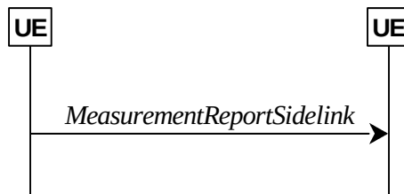
Figure 5.8.10.5.1-1: NR sidelink measurement reporting
