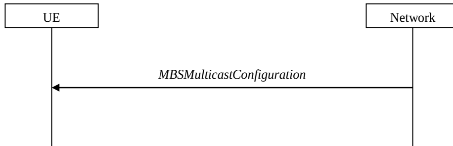
Figure 5.10.2.1-1: Multicast MCCH information acquisition
