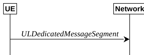
Figure 5.7.7.1-1: UL message segment transfer
