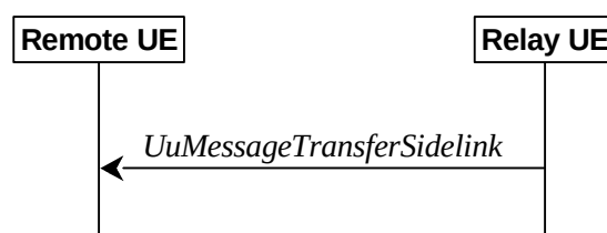
Figure 5.8.9.9.1-1: Uu message transfer in sidelink
