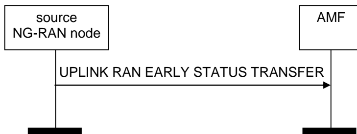
Figure 8.4.9.2-1: Uplink RAN Early Status Transfer
