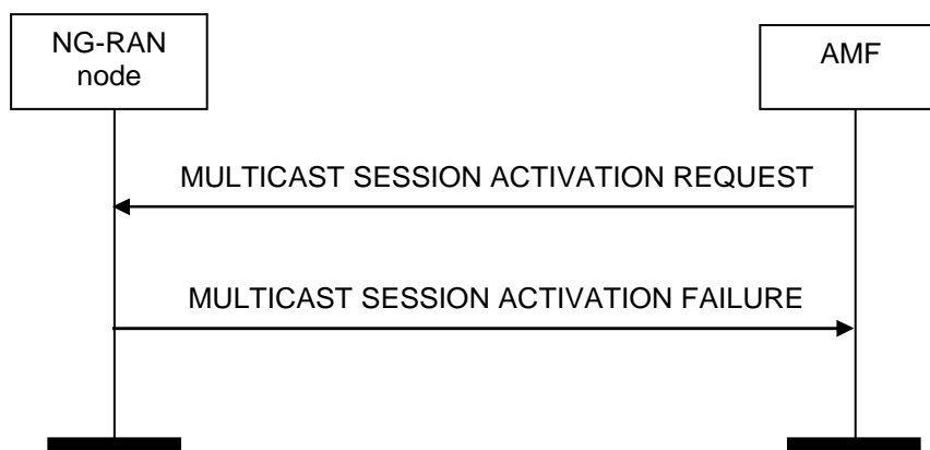
Figure 8.18.3.3-1: Multicast Session Activation, unsuccessful operation.
