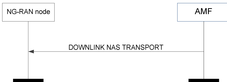
Figure 8.6.2.2-1: Downlink NAS transport
