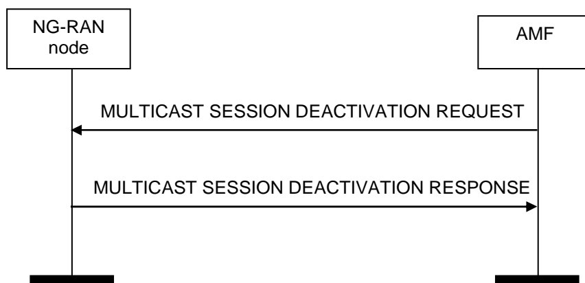
Figure 8.18.4.2-1: Multicast Session Deactivation, successful operation.
