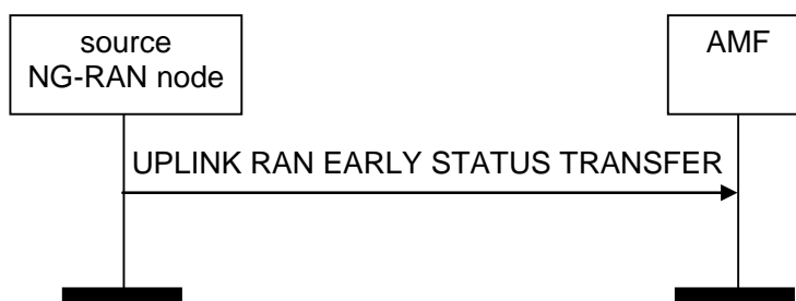
Figure 8.4.9.2-1: Uplink RAN Early Status Transfer
