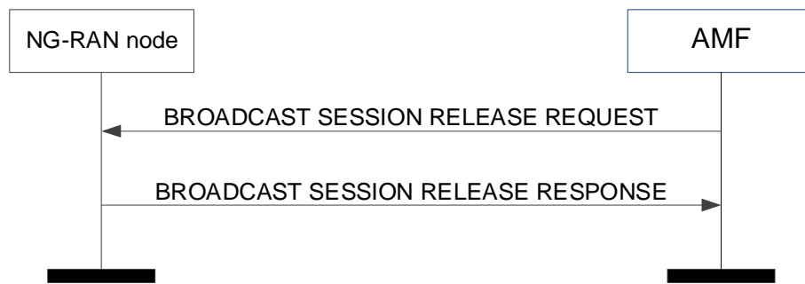
Figure 8.17.3.2-1: Broadcast Session Release, successful operation.
