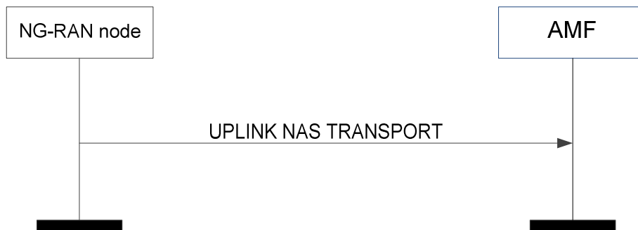
Figure 8.6.3.2-1: Uplink NAS transport
