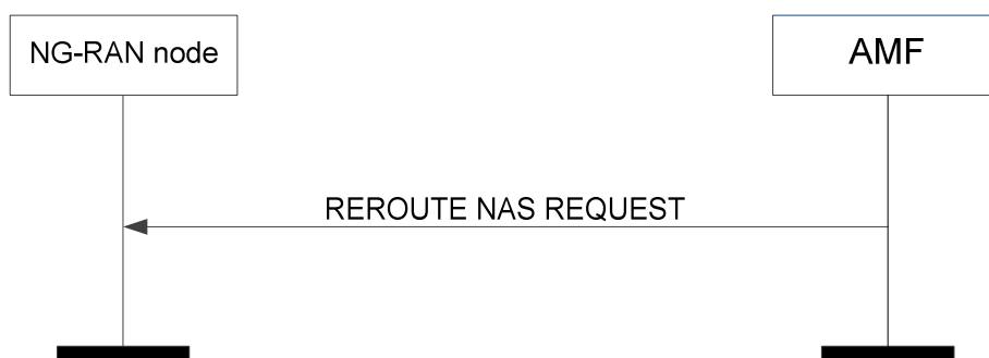
Figure 8.6.5.2-1: Reroute NAS request
