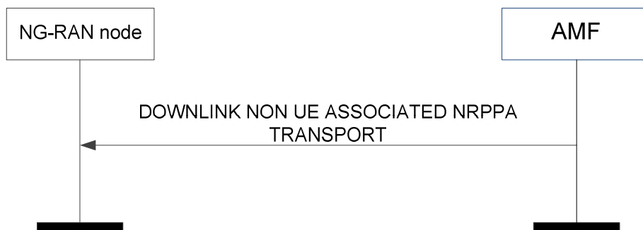
Figure 8.10.2.3-1: Downlink non UE-associated NRPPa transport
