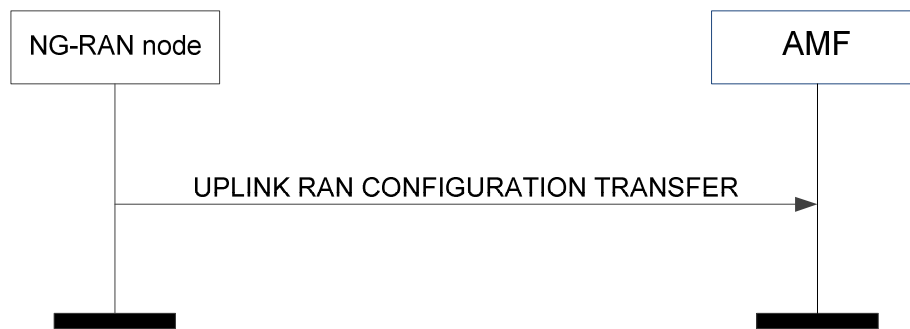
Figure 8.8.1.2-1: Uplink RAN configuration transfer
