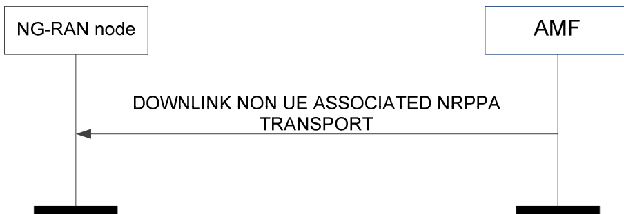
Figure 8.10.2.3-1: Downlink non UE-associated NRPPa transport
