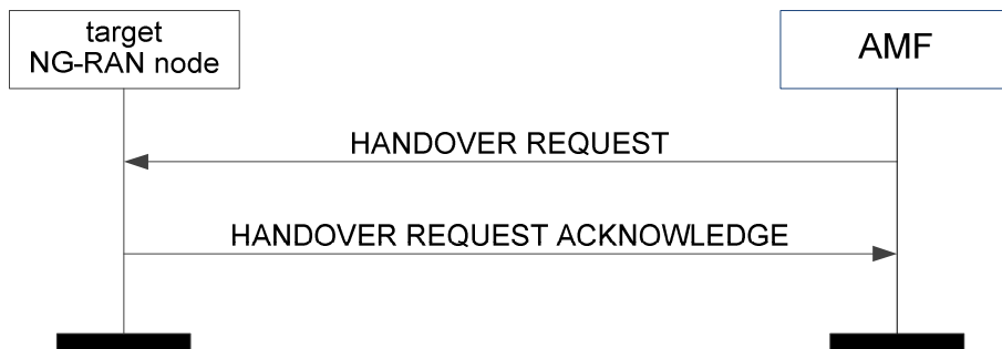
Figure 8.4.2.2-1: Handover resource allocation: successful operation
