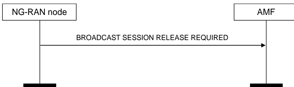
Figure 8.17.4.2-1: Broadcast Session Release Required, successful operation.
