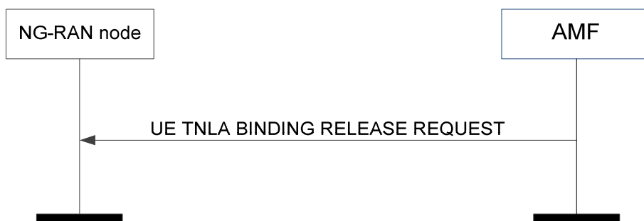
Figure 8.13.1.2-1: UE TNLA binding release request
