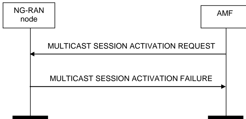
Figure 8.18.3.3-1: Multicast Session Activation, unsuccessful operation.
