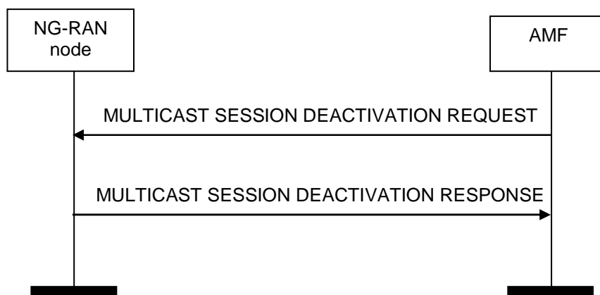
Figure 8.18.4.2-1: Multicast Session Deactivation, successful operation.
