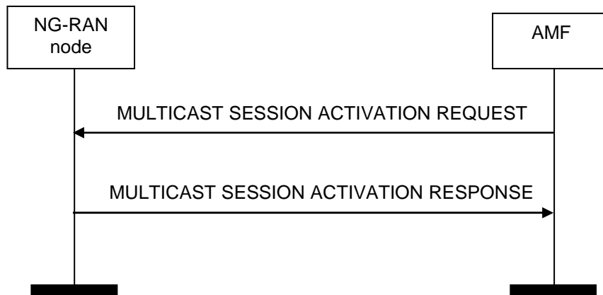
Figure 8.18.3.2-1: Multicast Session Activation, successful operation.
