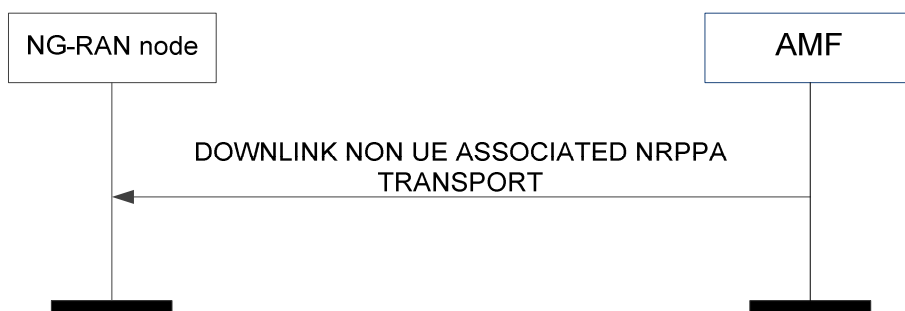
Figure 8.10.2.3-1: Downlink non UE-associated NRPPa transport
