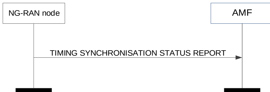
Figure 8.19.2.2-1: Timing synchronisation status report
