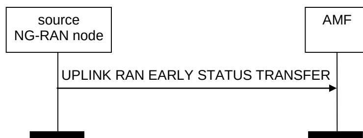
Figure 8.4.9.2-1: Uplink RAN Early Status Transfer
