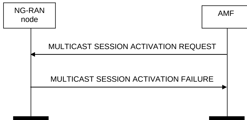
Figure 8.18.3.3-1: Multicast Session Activation, unsuccessful operation.
