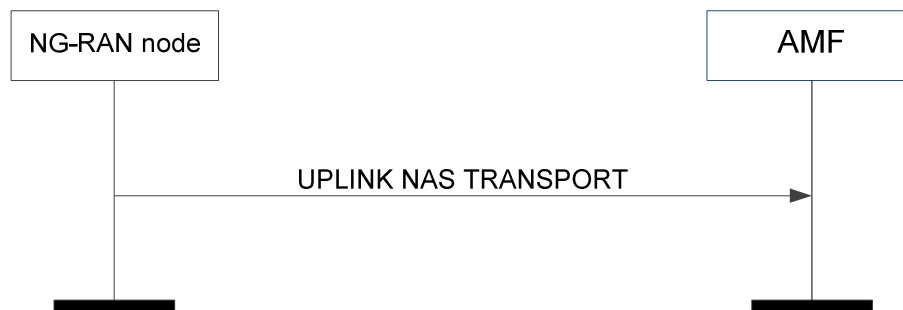
Figure 8.6.3.2-1: Uplink NAS transport
