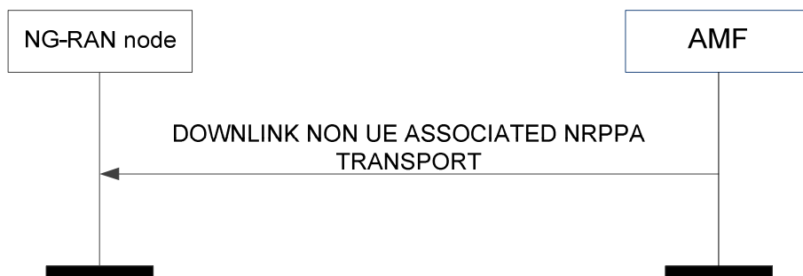
Figure 8.10.2.3-1: Downlink non UE-associated NRPPa transport
