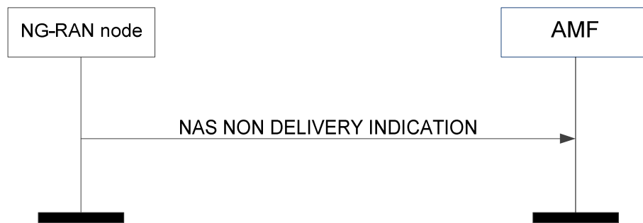
Figure 8.6.4.2-1: NAS non delivery indication
