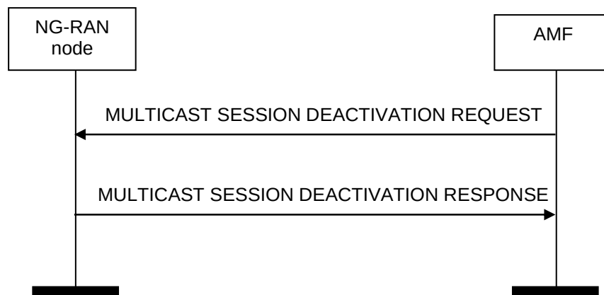
Figure 8.18.4.2-1: Multicast Session Deactivation, successful operation.
